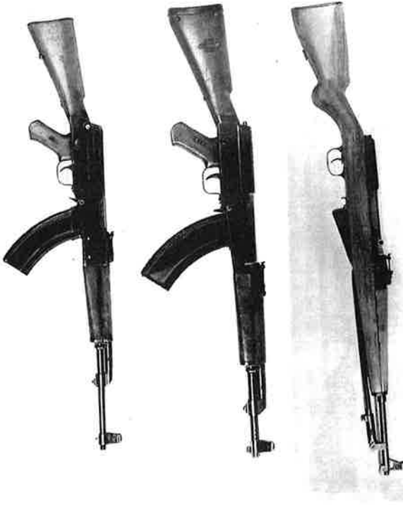
(Top) Figure 27. Experimental Model 1946 assault rifle (right side), designated SK #3 ( skaznyy vzor ) karabin , with bayonet folded. (Middle) Figure 28. Experimental AK-46, #1 (right side). (Bottom) Figure 29. Experimental AK-46, #2 (right side).
