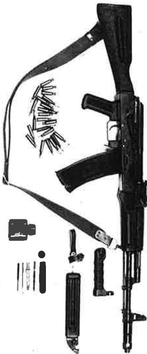
Figure 53. AK-74 with burststock folded and equipped with experimental muzzle brake with two side slots.
