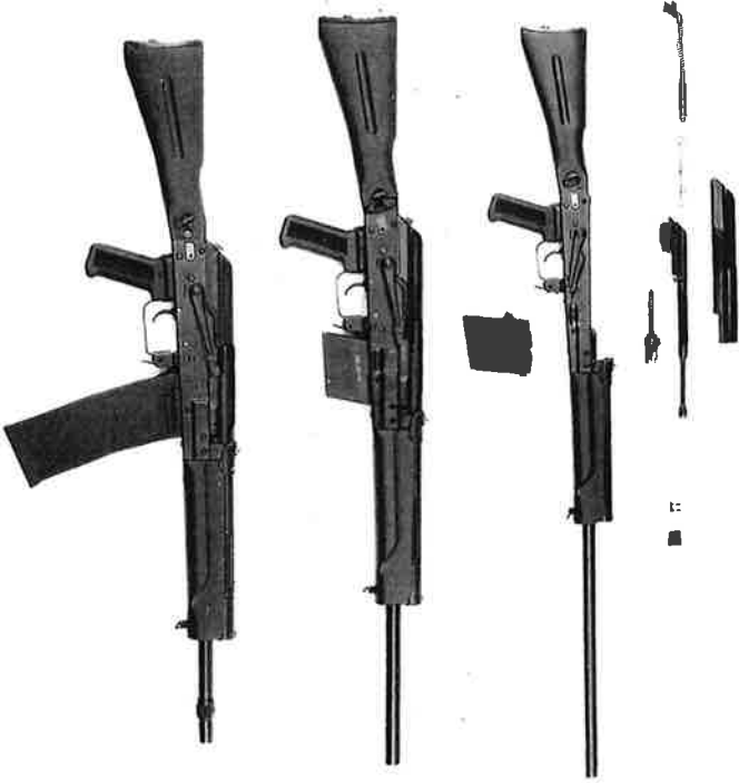
(Top) Figure 80, field-stripped Saiga-20S with buttstock extended. (Middle) Figure 81, Saiga-20 with a 4-round plastic magazine and a medium-length barrel. (Bottom) Figure 82, Saiga-20K (right side) with experimental 10-round magazine.
