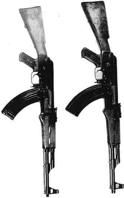
(Top) Figure 31. The AK-47 assault rifle, experimental version #3 (right side). (Bottom) Figure 32. AK-48 experimental version #1 (right side).
