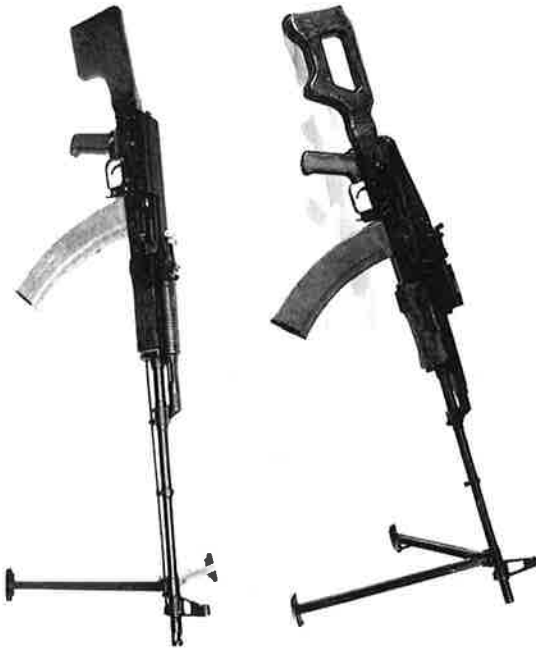
(Top) Figure 95. Experimental light machine gun with combined (alternating) feed from magazine and belt. (Bottom) Figure 96. The RPKS-74 Model 1974 light machine gun (right side) with folding buttstock.
