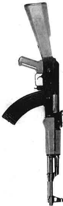
Figure 44, Model 1952 experimental AK assault rifle (right side) with AG-48 thermosetting plastic stock and forged and machined receiver.
