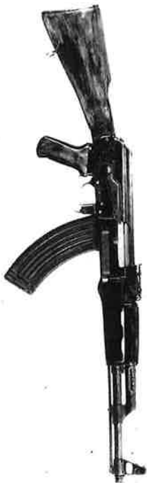
Figure 36. The AK-49 assault rifle. This model features the following modifications: the barrel extension is removed, the recesses were made right in the receiver, and the receiver is made by drop-forging and machining.
