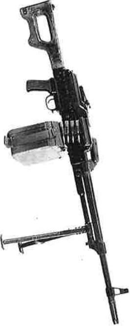
Figure 89. The PK Model 1961 unified machine gun with bipod.
