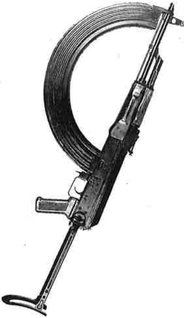
Figure 47. AKMs with experimental 100-round detachable stamped-and-welded magazine
