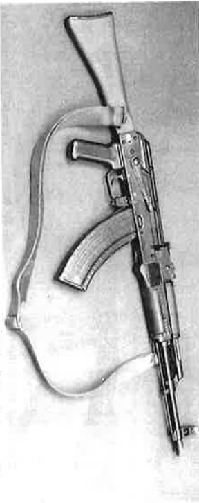
Figure 49. The AKMS assault rifle (right side) with experimental plastic folding stock and handguard and with stock extended.
