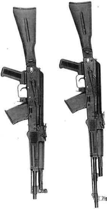
(Top) Figure 65. The KS semi-automatic-only rifle (right side), designed to the order of hunters and equipped with a 10-round magazine. (Bottom) Figure 66. The KSU short version of a carbine (right side) for professional hunting equipped with a 10-round magazine and with hushstock extended.
