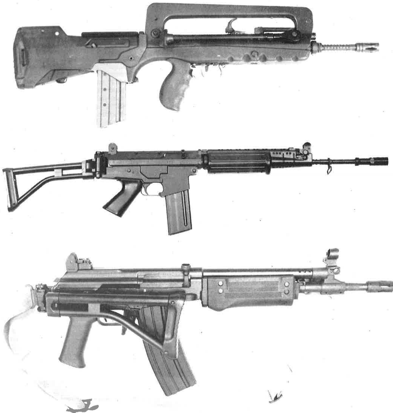
Top, the French contender in the NATO individual weapon trial—the 5.56 × 45mm FAMAS firing the US M193 cartridge; middle, Fabrique Nationale's 5.56 × 45mm FNC barreled to fire the SS109 projectile (1-in-7 barrel twist); bottom, the Israeli Military Industries 5.56 × 45mm Galil, designated the MN1—The Netherlands' entry in the individual weapon trials.
