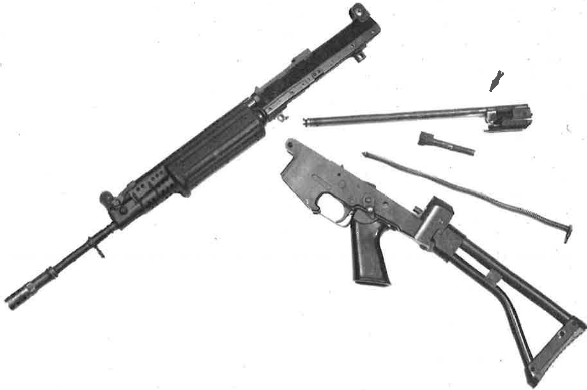
The Fabrique Nationale FNC field stripped. Note similarity of the bolt and bolt carrier assembly to that of the Kalashnikov weapons.
