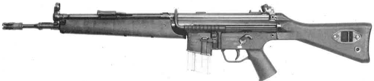
The Heckler & Koch G41. Note the longer barrel, redesigned handguard, modified lower receiver, carrying handle, and M16-type magazine.
