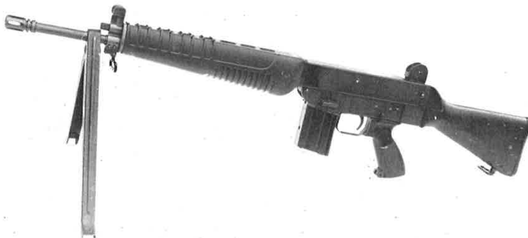
Chartered Industries of Singapore 5.56 × 45mm SAR 80 assault rifle, which evolved from the AR-18.
