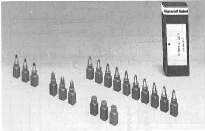
The 1982 family of 4.7 × 21mm caseless cartridges. Top row, ball projectiles; bottom row, tracers, plastic training rounds, and blanks.
