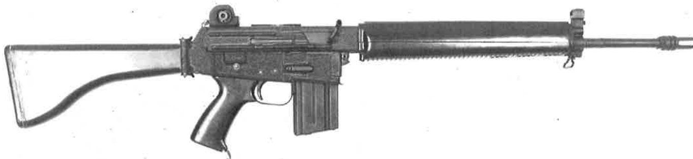
Sterling Armament Company's AR-18 5.56 × 45mm rifle.
