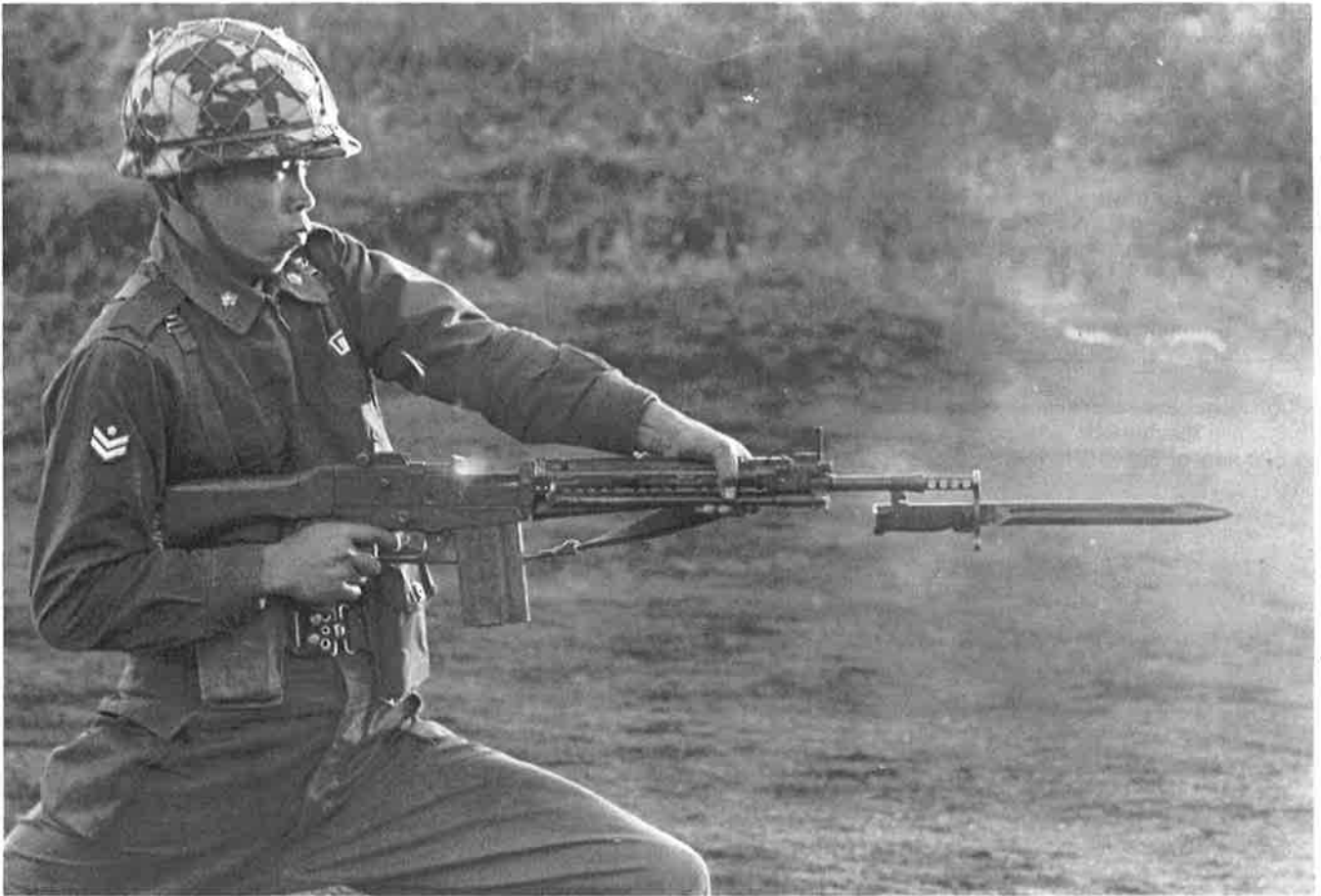
The 7.62mm Japanese Type 64 rifle as manufactured by Howa. This rifle was designed to fire a reduced charge version of the 7.62 × 51mm NATO cartridge.
