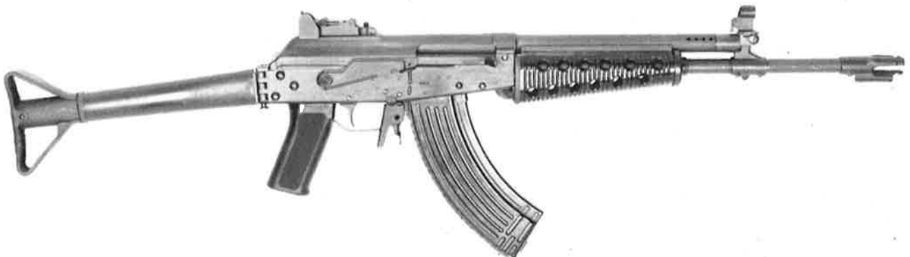
Finnish copy of the AKM manufactured by Valmet Oy Defense Equipment Group. Note that this M62-76 rifle has a side folding stock.
