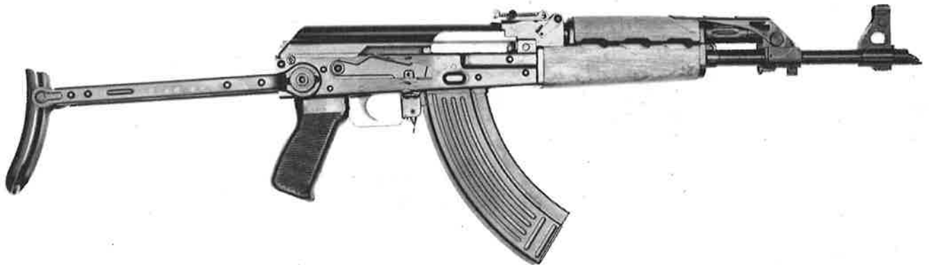
Yugoslav 7.62 x 39mm M70AB with an AKM pressed sheet metal receiver.
