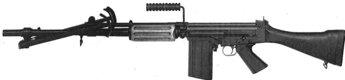
Standard FN heavy barrel FAL, designated the FALO by the FN factory. (FALO is an acronym meaning FAL lourd , FAL heavy.)
