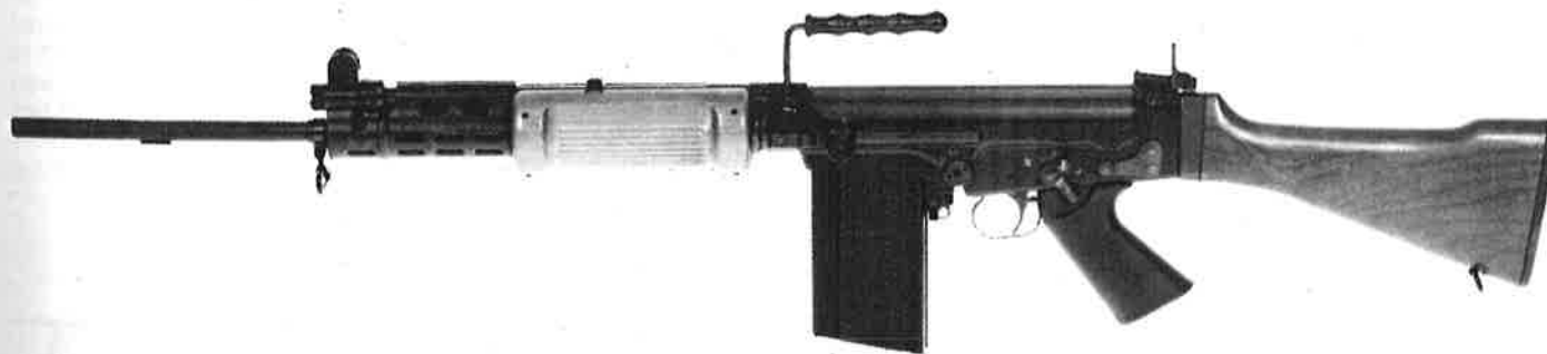
Israeli FAL. All parts except the receivers were manufactured by Israeli Military Industries. FN manufactured the receivers. Note the strengthened front sight and gas cylinder assembly and the modified handguard. In this model the cocking handle can be used as a forward bolt assist.
