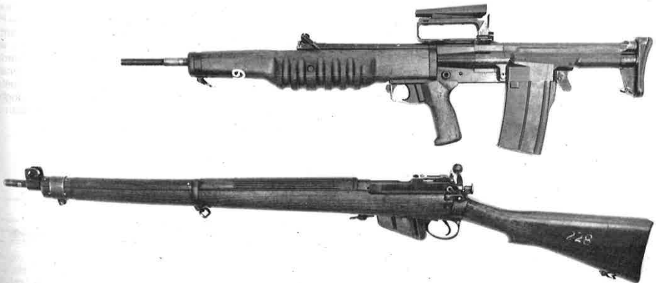
Top: Rifle, .280 E.M.2. Bottom: Rifle No. 4 Mark 1. The No. 4 Rifle fired an 11.3-gram (174-grain) projectile at 751 m/s (2465 f.p.s.) from a 592mm (23.3-inch) barrel; while the E.M.2 fired an 8.4-gram (140-grain) projectile at 736 m/s (2415 f.p.s.) from a 622mm (24.5-inch) barrel. Overall length of the E.M.2 was kept short by its bull pup design. The magazine and receiver group are to the rear of the pistol grip, thus permitting the use of a full length barrel in a shorter weapon: E.M.2 914mm (36 inches) vs No. 4 1079mm (42.5 inches).
