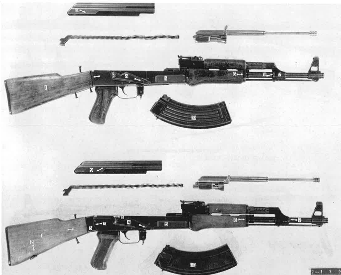
Second (bottom) and third (top) versions of the AK47. Note differences indicated by numbers in the photograph.
