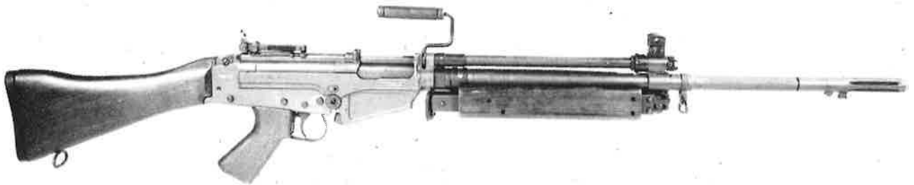
Canadian-made C2 heavy barrel version of the FN FAL.
