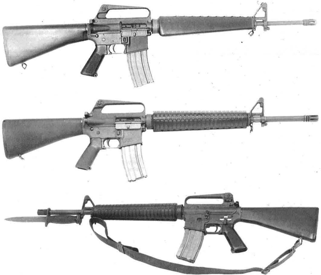
Top, standard 5.56 × 45mm (M193) M16A1 rifle; middle, Colt proposal for product-improved M16A1 (heavier barrel, improved handguards and butt stock); bottom, 1982 candidate PIP M16A1 with additional features of improved rear sight and three-shot burst control.
