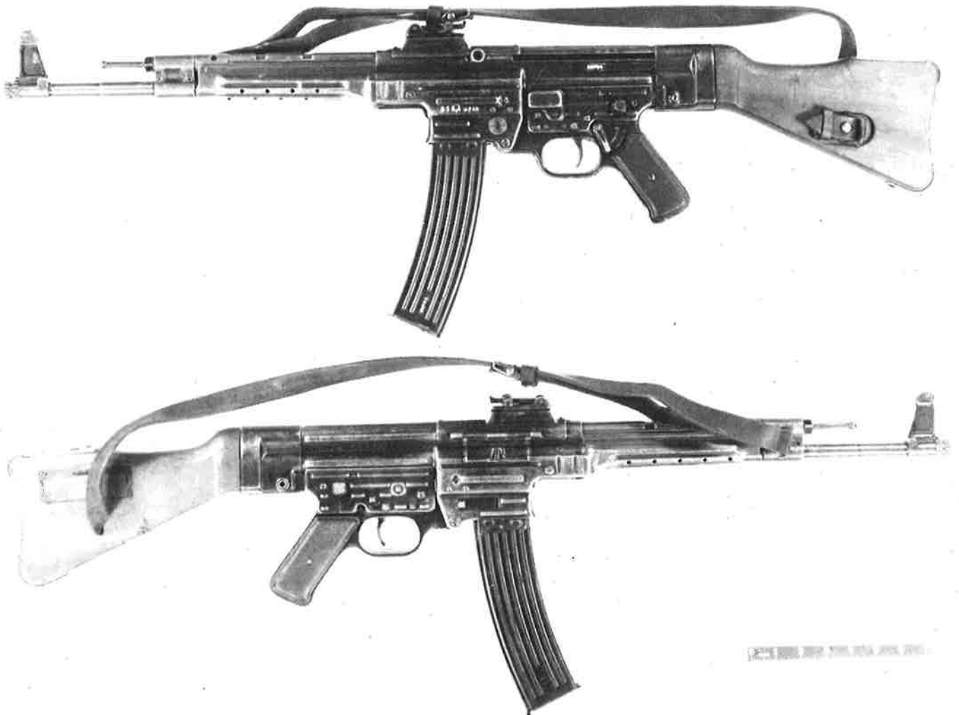
Typical Sturmgewehr , the German MP44, which fired the 7.92 × 33 cartridge.
