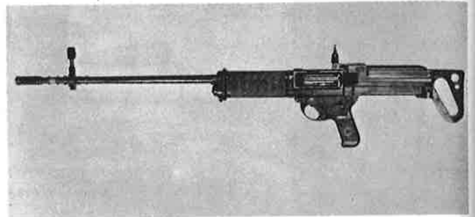
Prototype Waffenfabrik Bern 7.5mm Assault Rifle. Fired standard 7.5 × 55.5mm cartridge.
