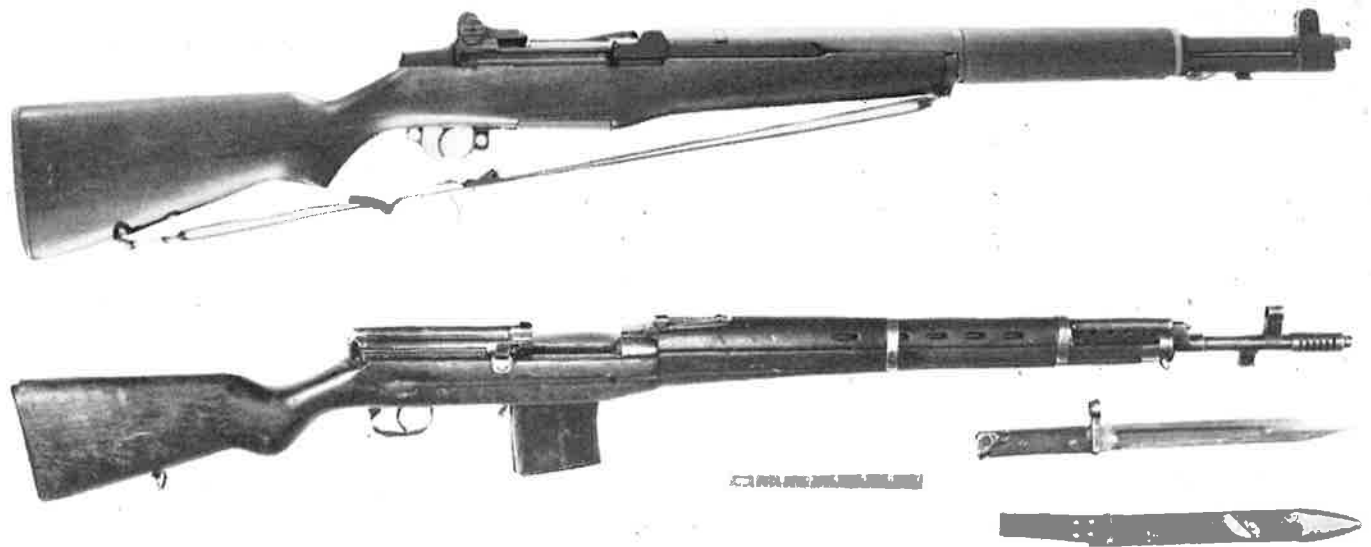
Top, US Rifle, Caliber .30, M1—eight-shot clip; bottom, USSR Samozariadnyia Vintovka Tokareva Obrazets 1938G (SVT-38) 7.62 × 54Rmm—ten-shot magazine. The M1 Rifle was produced from 1936 to 1945 and again during the Korean conflict of the 1950s. The SVT-38 was modified in 1940, and both semiautomatic (SVT-40) and selective fire (AVT-40) versions were produced during World War II.
