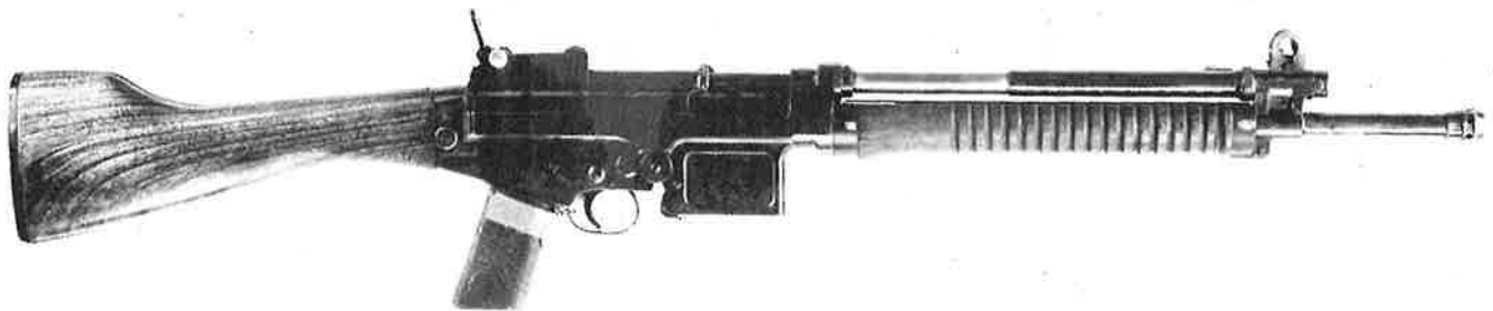
Early FAL prototype chambered for the 7.92 × 33mm Kurz cartridge.
