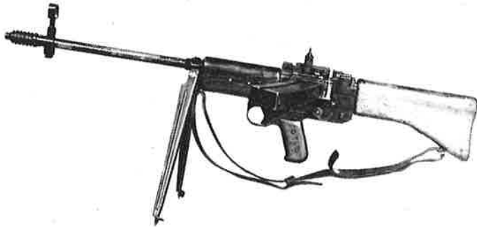
Prototype Waffenfabrik Bern 7.5mm Short Rifle. Fired experimental short cartridge.
