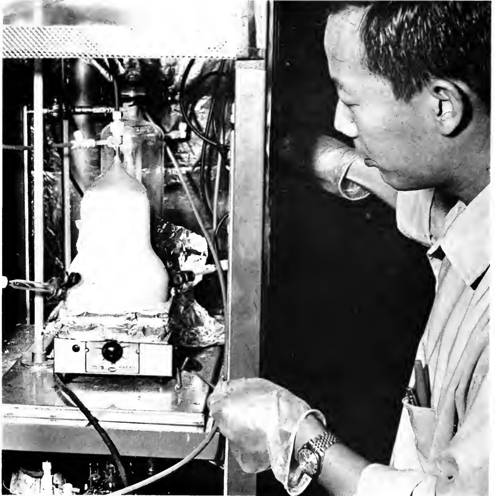
DOPING A SILICON WAFER IN THE INTEGRATED CIRCUITS LABORATORY Department of Electrical Engineering
