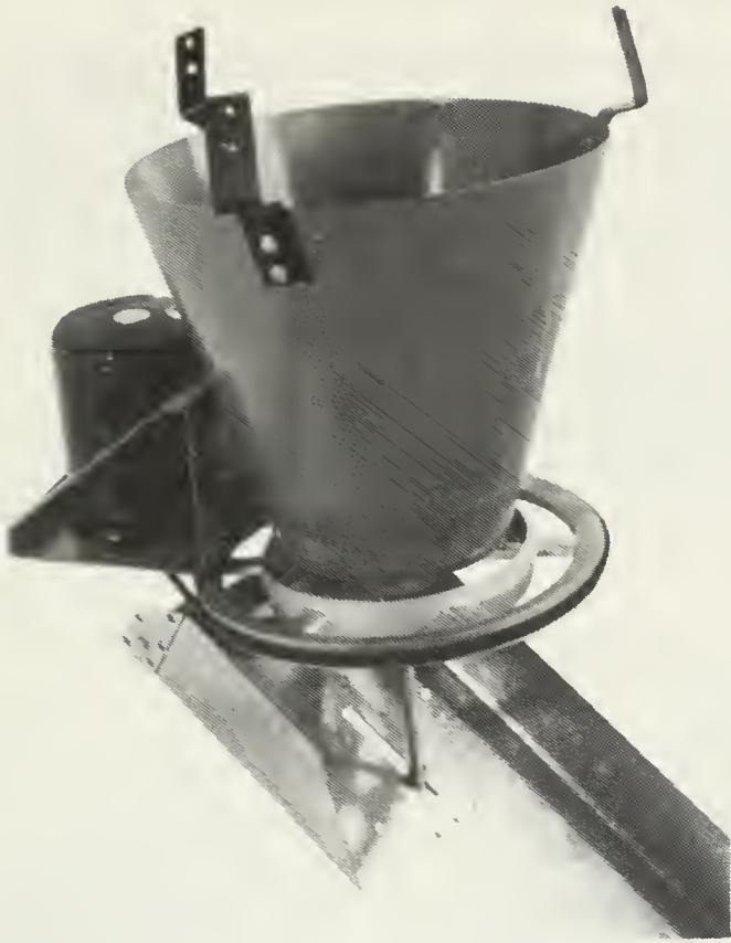
electrically operated tilting-pan type, 5-11 m bins
