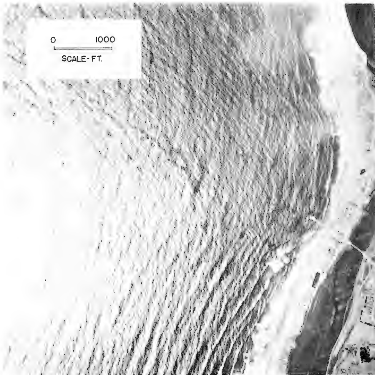
Figure 30.—Wave refraction at Moss Landing. Note the "flat" water at the end of the pier where the Monterey Canyon approaches the shore. Compare complicated refraction pattern with hydrography in figure 7.
