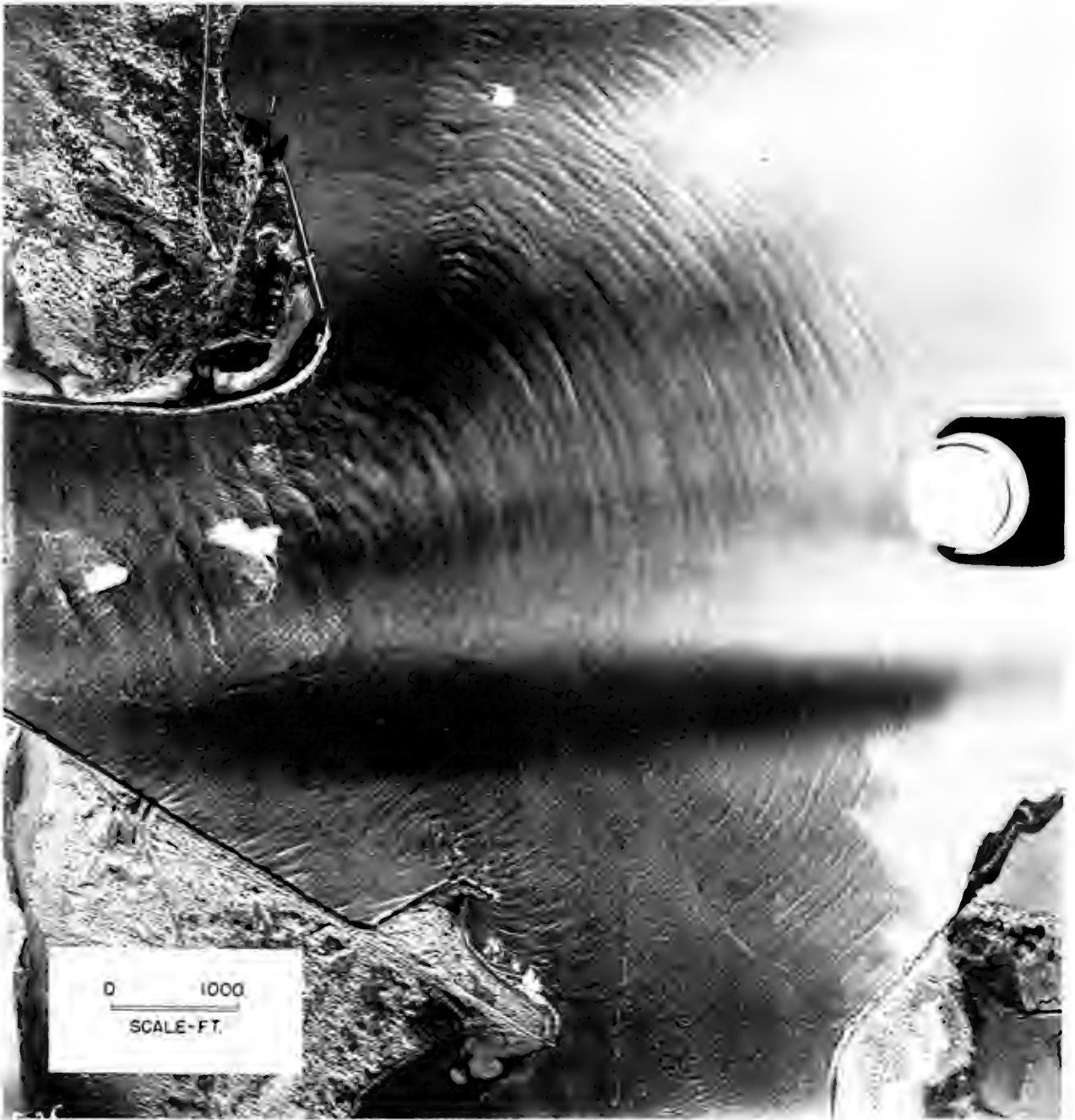
Figure 26.—Wave refraction inside Humboldt Bay. Note wave fronts crossing at shoal in upper right-hand corner. At this point the waves augment each other and break.
