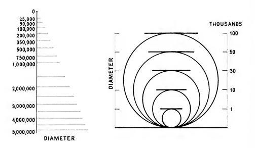
Two Methods of Making a Scale to Indicate What the Area of a Circle Represents by Measuring Its Diameter.
