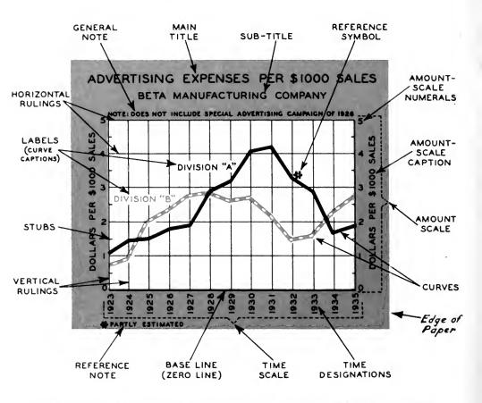
The arrow and designation "Edge of Paper" have been added to the original in order to indicate that the outside line is not a frame. The author believes it is undesirable to put a frame line around a chart because of the possibility of that line being falsely interpreted as a zero line.
