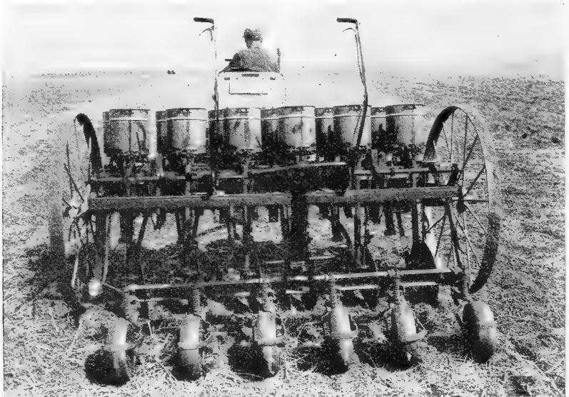
FIGURE 2.—A planter-type grass drill designed and constructed at Woodward, Okla., showing seed being broadcast from the front row of boxes and drilled shallow from the rear. Note the protective crop residue on this seedbed of disked Sudan grass stubble.
