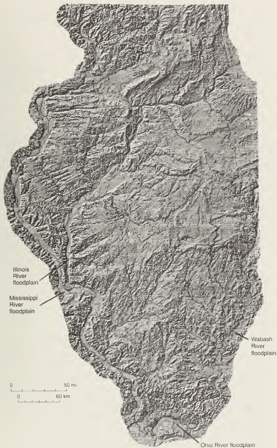
12 Shaded relief map of Illinois and parts of adjacent states. Nearly flat floodplains of the major rivers stand out in contrast to the variable relief of the uplands. (Computer-generated map from the Illinois Geographic Information System. Mapping derived from U.S. Geological Survey Digital Elevation Model data at 1:250,000 scale.)
