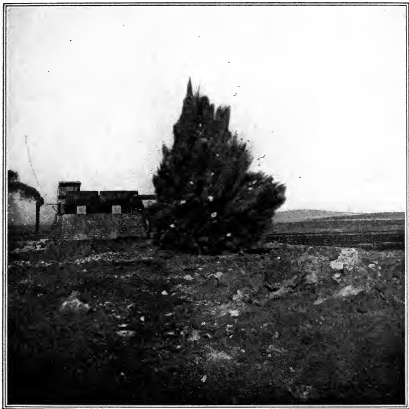
FIG. 6.—Explosion in caliche bed.
