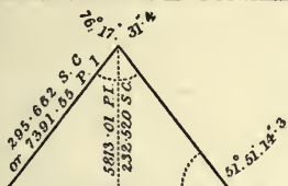
DIRECT VERTICAL SECTION OF GREAT PYRAMID.
