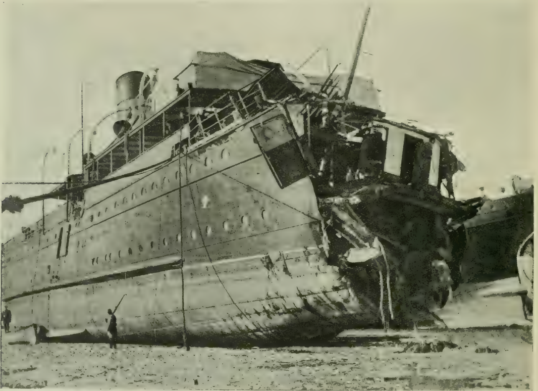
The Torpedoing of the Channel Steamer Sussex : view of the vessel beached at Boulogne, showing how the bows were blown clean off by the explosion
