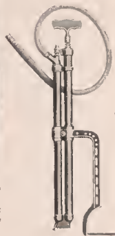
The pump sprayer above is designed to be used with a pail of liquid. The two tubes go inside the pail and an outside foot-piece holds them in place while operating. Courtesy D. B. Smith & Co.
