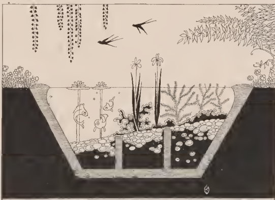
A cross-section of the concrete-lined pool shows the sloping arrangement of the soil and the partitions to hold it in place
