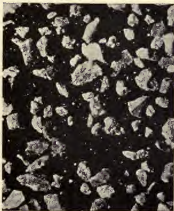
FIG. 4.—EMERY, No. 60. 20 DIAMETERS
