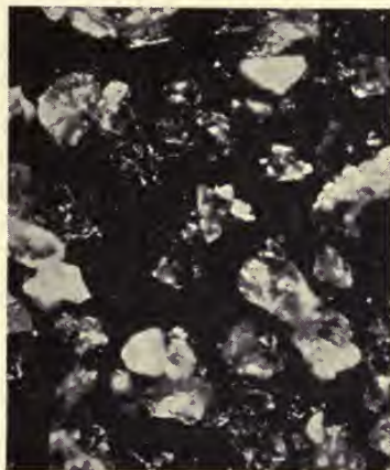
FIG. 7.—ALUNDUM, No. 60. 20 DIAMETERS
