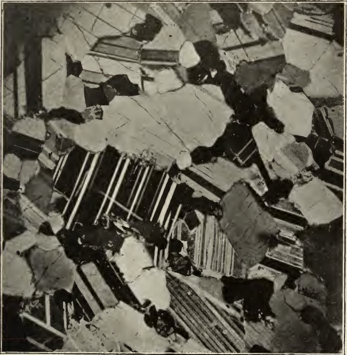
Anorthosite from New Glasgow, P.Q. Microphotograph between crossed nicols. × 28 diam.
