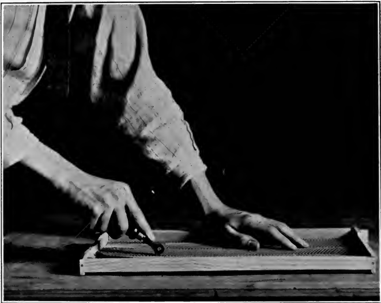
Fig. 19. Embedding Wire in Foundation.
