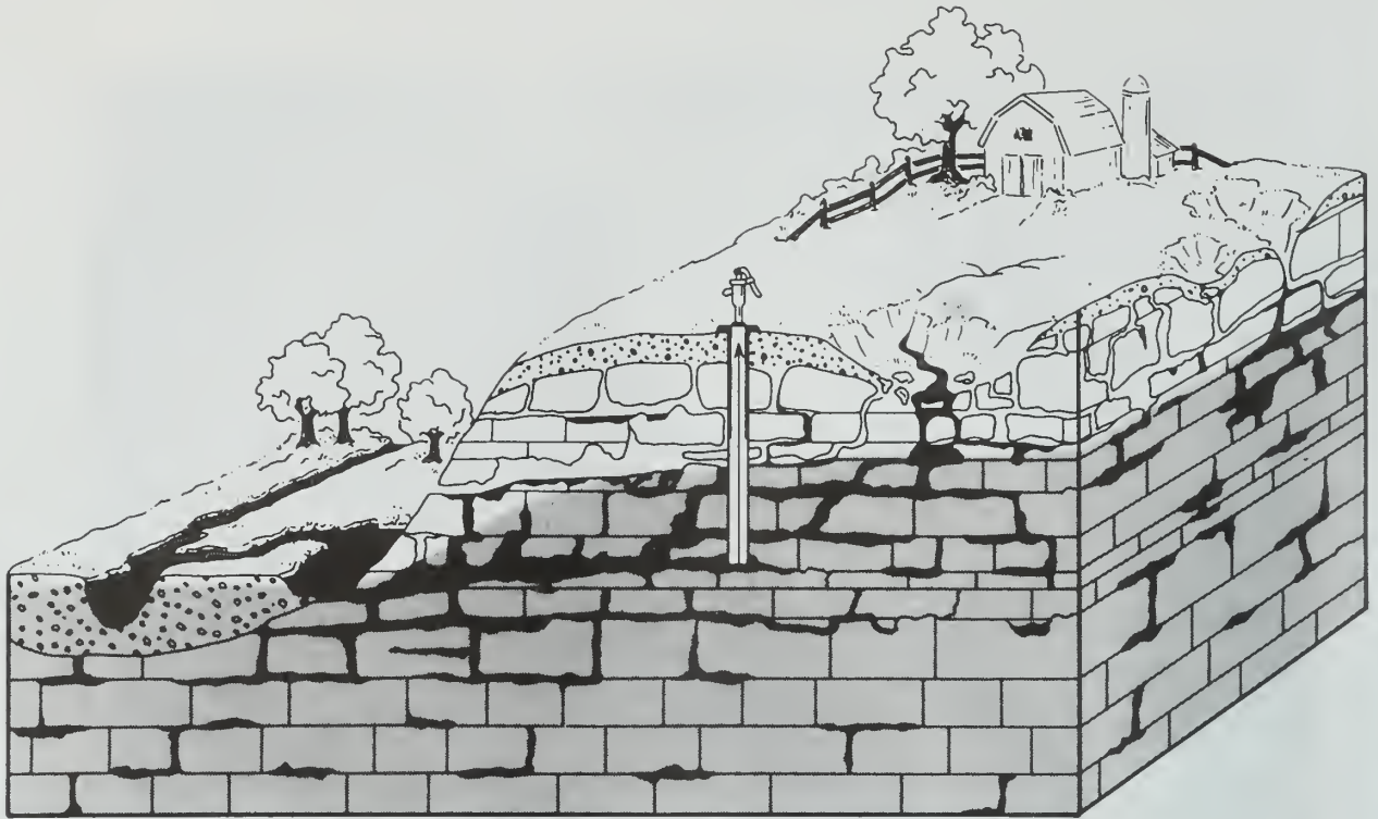
Figure 20 Karstification in an area of jointed limestone bedrock (Hallberg et al. 1984).
