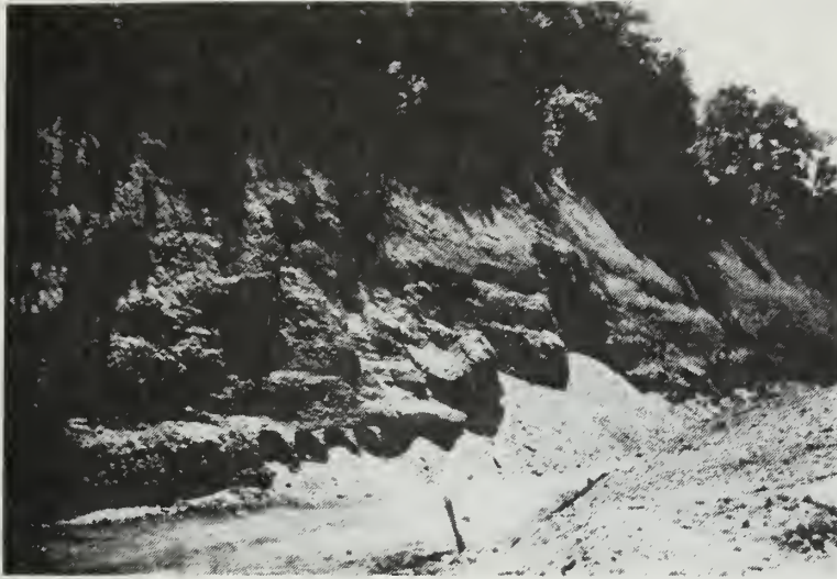
Figure 5. Lee Coal Company high-wall shows auger-mining holes in Danville (No.7) Coal partly covered by face slumping. (Reinertsen, 1976.)
