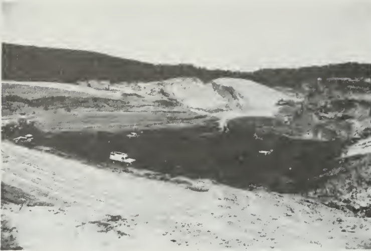
Figure 6. View to east of Lee Coal Company strip mine in No. 7 Coal. Note rough spoil piles and steep highwall face to right. (Reinertsen, 1976).
