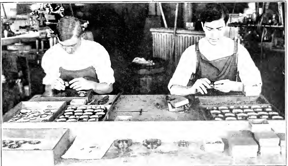
PUTTING TOGETHER THE SHUTTERS.
