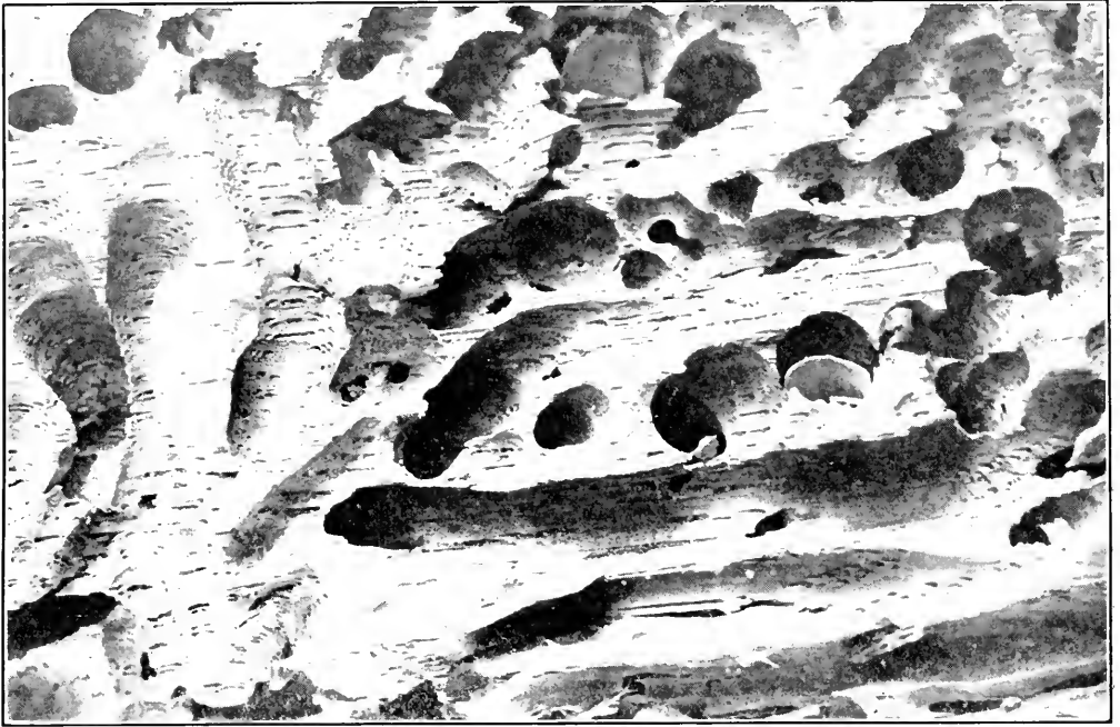
A VIEW OF TEREDO BORINGS UNDER A POCKET MICROSCOPE.
