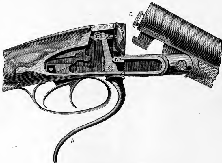
Mechanism of Murcott's Hammerless Gun.
