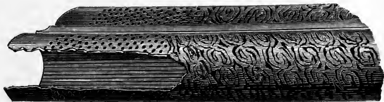
Grooved and Perforated Shot Barrel.
