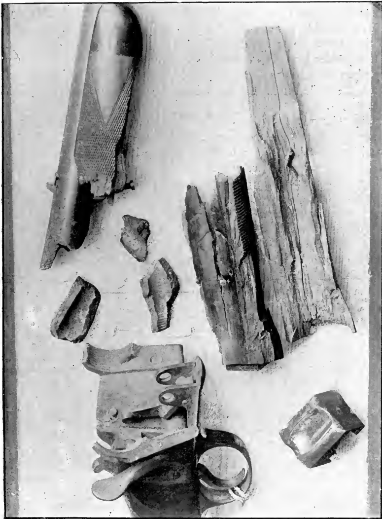
"Express" Rifle burst with Fine-grain Powder.
