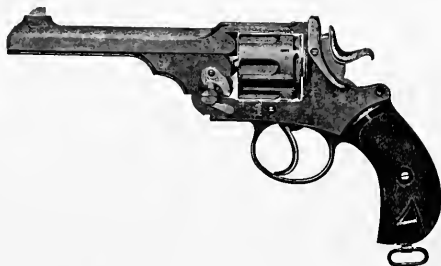
FIG. 6.—Webley "W. G." Army Model Revolver. Six shots; 6-inch barrel; weight, 2 lb., 8 oz.; .455 cal.
