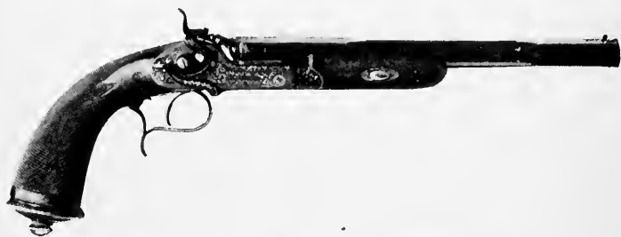
FIG. 15. — Gastinne-Renette Pistol. 10\frac{3}{16} -inch barrel; weight, 2 lb., 6 oz.; .44 cal.
