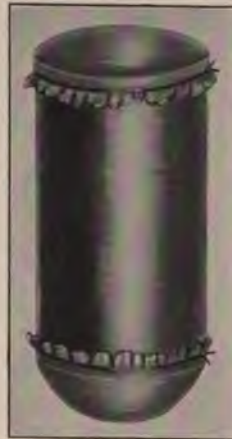
FIG. 7.—A Vertical Cylinder closed at either End by an Elastic Diaphragm and Filled with Fluid.
