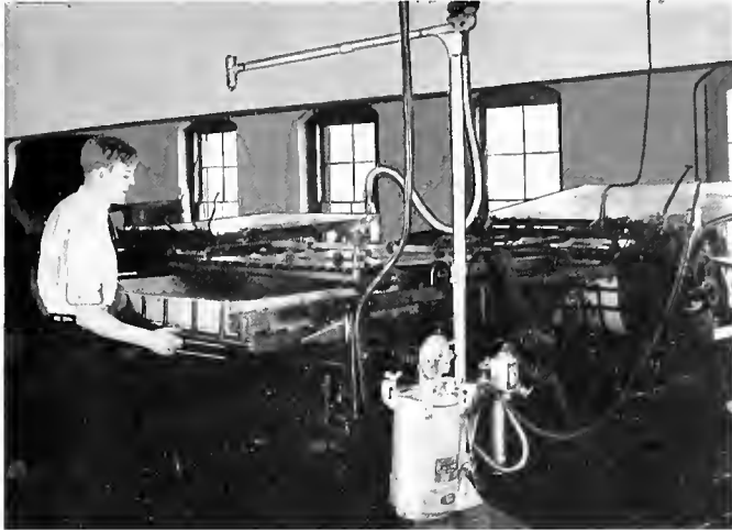
The ingenious spray gun, shown in foreground, prevents ink smears as your pages speed through the press.
