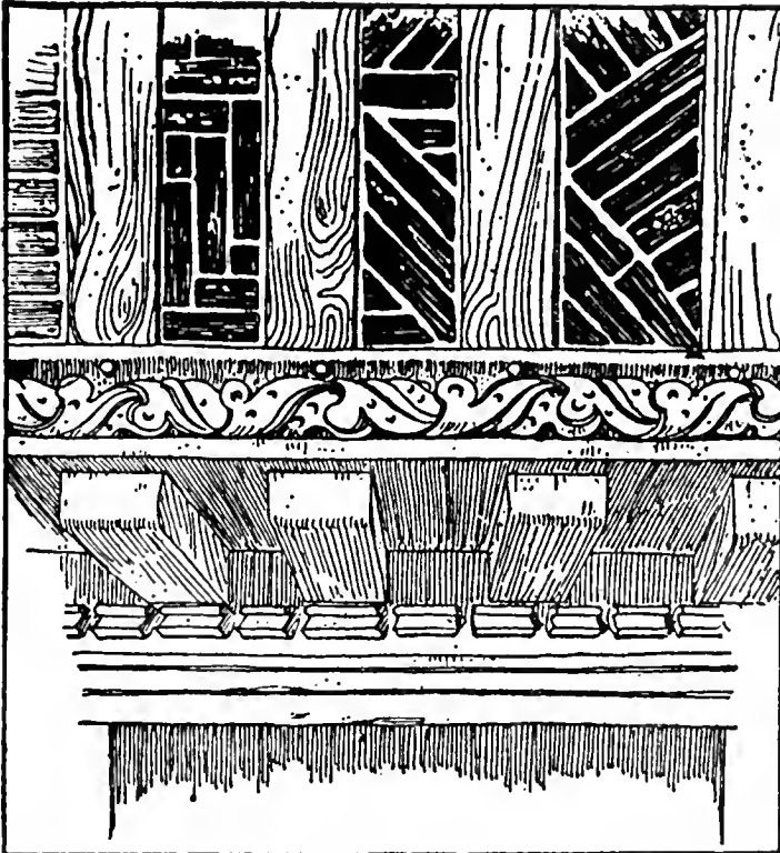
Brick was frequently used as the material for filling in between the timbers, laid up in a variety of patterns
