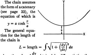
where the value of  $\frac{dy}{dx}$ , obtained by differentiating the equation of the catenary, is
