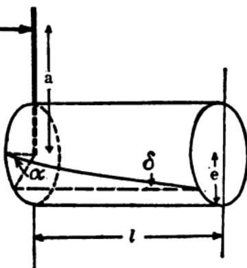
$$\text{Horsepower} = \frac{2 \pi PaN}{33,000 \times 12}$$
