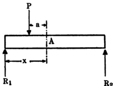
under Beam Loadings) is equated to  $\frac{pI}{e}$ . The term  $\frac{I}{e}$ , called the section modulus, may be obtained from the table of standard sections of beams. The value of  $p$  must not exceed the maximum allowable stress per unit area for the material of the beam. The **maximum allowable stress** equals the ultimate strength divided by the factor of safety.
