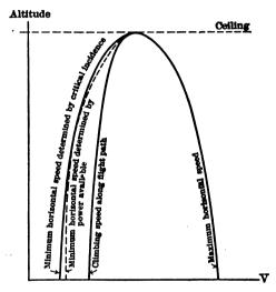
the maximum horizontal speed does decrease as the altitude increases. The value of n also decreases, though only slightly. Hence S decreases and in general e falls off, so that the "power available" curve is decidedly lowered at high altitudes. Eventually there is reached an altitude (ceiling or absolute ceiling) at which only one speed is possible and above which flight is impossible.
