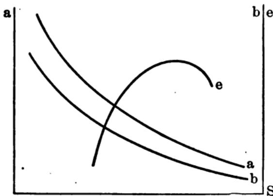
The values of  $a$ ,  $b$ , and  $c$  are usually determined from wind tunnel experiments, and plotted on the base,  $S = \frac{V}{nD}$ , which may be called the **effective pitch ratio** and is equal in homologous units to  $p(1 - s) \div D$ , where  $p$  = pitch,  $s$  = slip.
