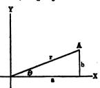
cation by the imaginary unit, j, revolves a quantity through 90 degrees, in counter-clockwise direction.
