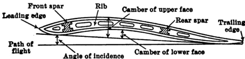
ponents of an approximately normal force acting at the **center of pressure**. This force is mainly a suction on the upper face. The position of the center of pressure varies with the incidence.
