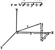
II. The direction cosines of the line from the point (x, y, z) to the origin are:
