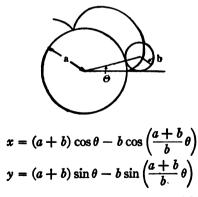
where a is the radius of the fixed circle, and b the radius of the rolling circle.
