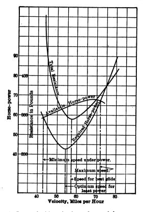
speed (lower incidence) than does minimum power required. The latter condition is the condition of maximum endurance (hours in the air). Since W(=L) decreases during flight, the speeds of least power and
