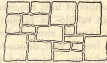
FIG. 31.—Random Range Laid in Level and Broken Courses.
