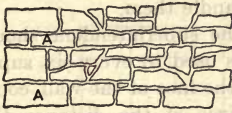
FIG. 30.—Broken Rubble, with Bond Courses AA Extending through the Wall, Makes a Very Strong Wall.
