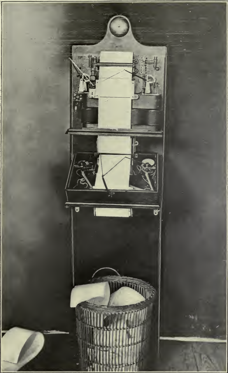
167. Telautograph, with Cover Removed to Show the Working Parts.
