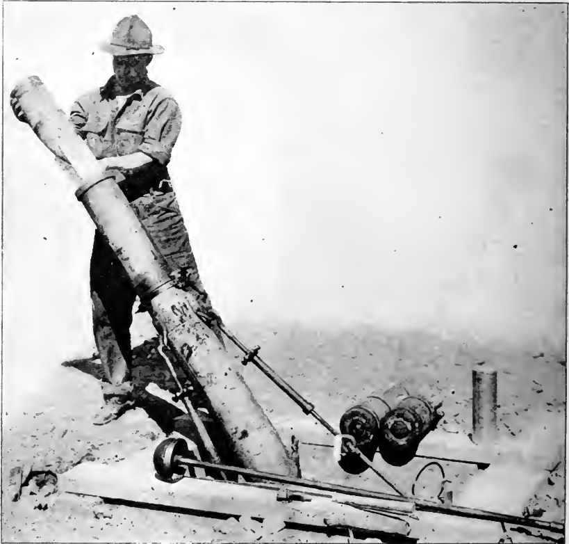
METHOD OF LOADING TRENCH MORTAR.
