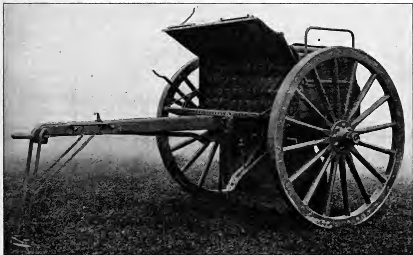
FRONT VIEW, SHOWING DOOR SWUNG UPWARD EXPOSING AMMUNITION.
