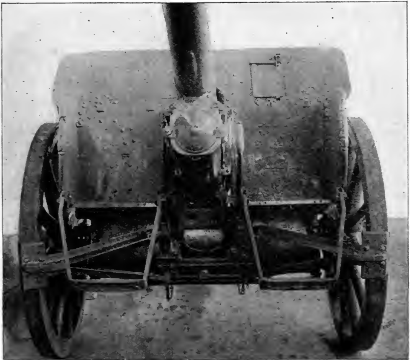
FRONT VIEW, SHOWING BRAKES AND TRAVELING LOCK.
