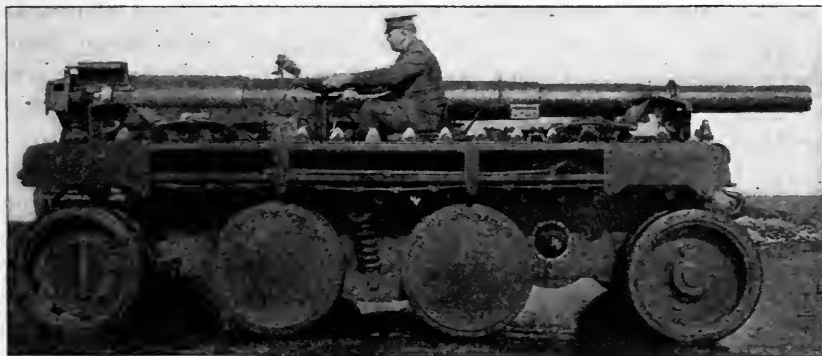
SIDE ELEVATION OF MOUNT IN TRAVELING POSITION.
