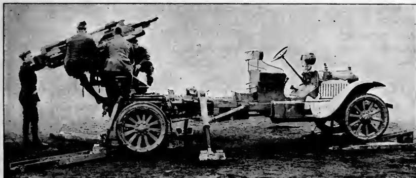
VIEW SHOWING TRUCK MOUNT IN ACTION.
