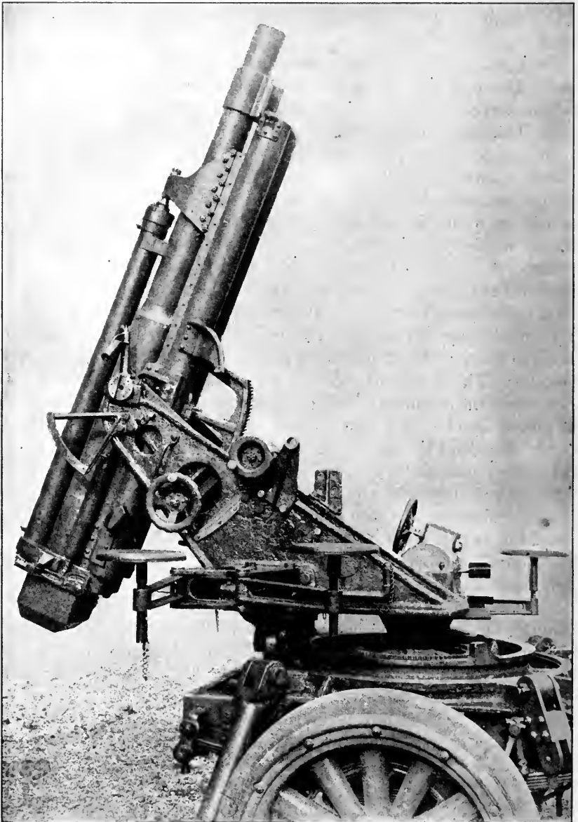
GUN MOUNT SHOWING GUN AT MAXIMUM ELEVATION.
