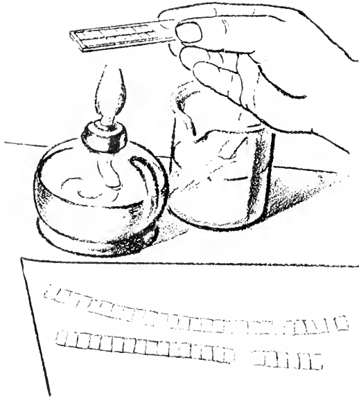
Fig. 117. Warming the flooded ribbons to flatten them.
