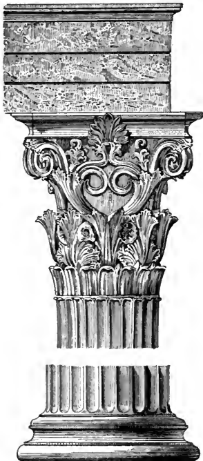
FIG. 101.—Base, capital, and architrave of monument of Lysicrates. (Borrmann, Geschichte der Architektur , I, Fig. 97.)
