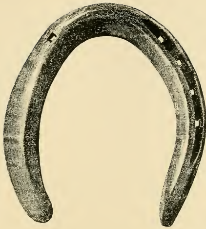
FIG. 296.—Concave feather-edged hind shoe, partially fullered Made in concave tool, from old shoes or from \frac{3}{4} \times \frac{1}{2} inch iron.
