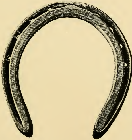
FIG. 210.—Fullered fore shoe for hack. Made from \frac{1}{2} inch \times \frac{5}{16} iron.
