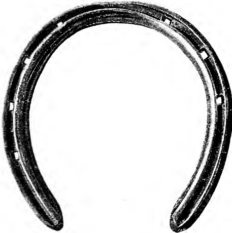
FIG. 227.—Concave fullered fore shoe (for steeplechasing). Made from \frac{3}{4} \times \frac{3}{8} inch iron.
