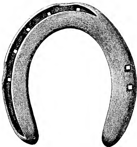
FIG. 292.—Fullered seated feather-edged fore shoe. For harness or riding. Made from \frac{7}{8} \times \frac{1}{2} inch iron.
