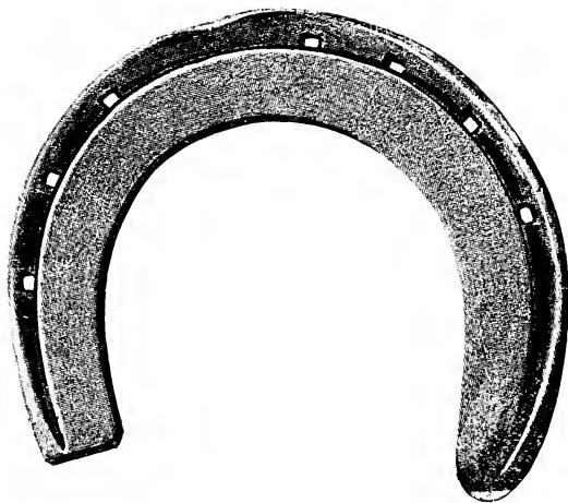
FIG. 370.—Three-quarter fullered seated fore shoe. Made from 1 \cdot \frac{1}{2} inch iron.
