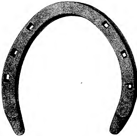
FIG. 223.—Charlier hind shoe, made from Charlier steel, 7-16th inch square.
