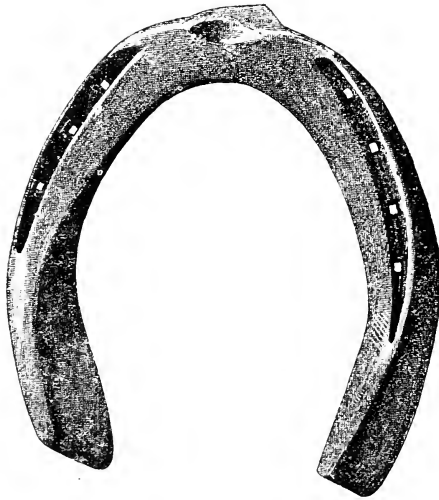
FIG. 391.—Fullered wedge-heeled hind shoe (for harness horse). Made from \frac{3}{4} - \frac{1}{2} inch iron.
