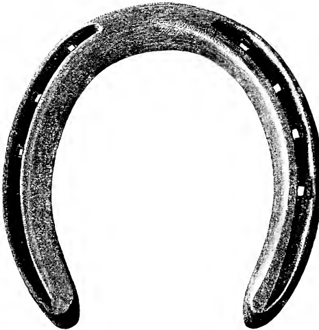
FIG. 217.—Concave partially-fullered, 'dub-toed' fore shoe. Made from \frac{3}{4} \times \frac{1}{2} inch iron.
