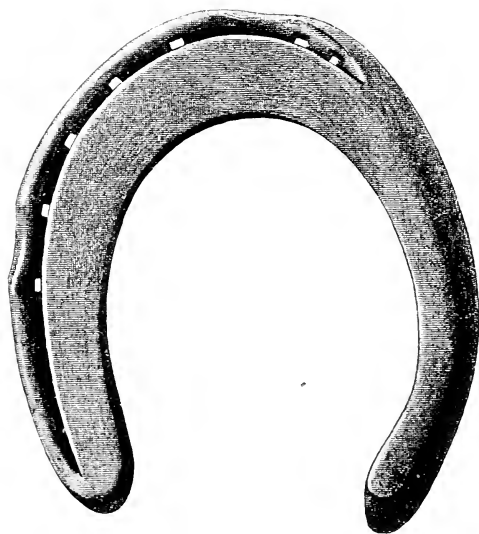
FIG. 293.—Fullered seated feather-edged fore shoe. Made from 1\frac{1}{8} \times \frac{1}{2} inch iron.
