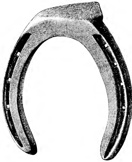
FIG. 276.—Fullered hind shoe for harness horse which forges and wears wall of hind foot. Made from \frac{3}{4} \times \frac{1}{2} inch iron.
