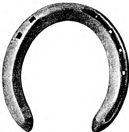
FIG. 218.—Concave fuller, feather-edged fore shoe. Made of \frac{3}{4} \times \frac{1}{2} inch iron in concave tool.
