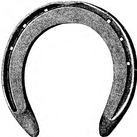
FIG. 396.—Fullered seated fore shoe. Made from \frac{7}{8} \times \frac{1}{2} inch iron.
