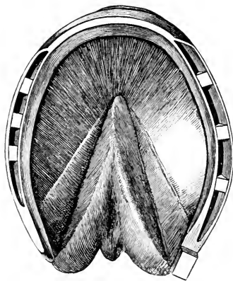
FIG. 214.—Hind shoe for hunter. The toe is rounded and set back to prevent overreach. The sole has been pared so as to cause the bar to appear as if extending to the point of frog.
