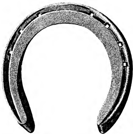
FIG. 211.—Fullered seated fore shoe with thick heels. Made of \frac{5}{8} \times \frac{5}{8} inch iron.
