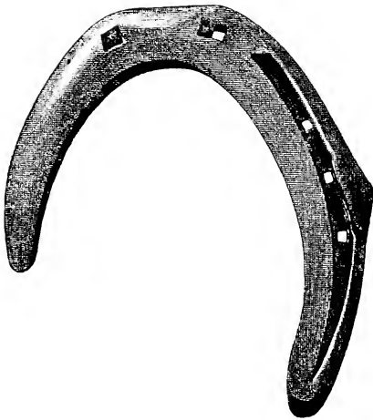
FIG. 300.—Three-quarter partially fullered hind shoe. Made from old shoes, steel, or \frac{3}{4} \times \frac{1}{2} inch iron.
