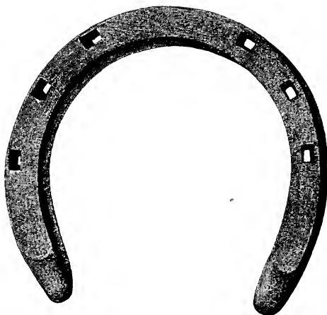
FIG. 219.—Stamped fore shoe. Made from Charlier steel \frac{7}{16} inch square.
