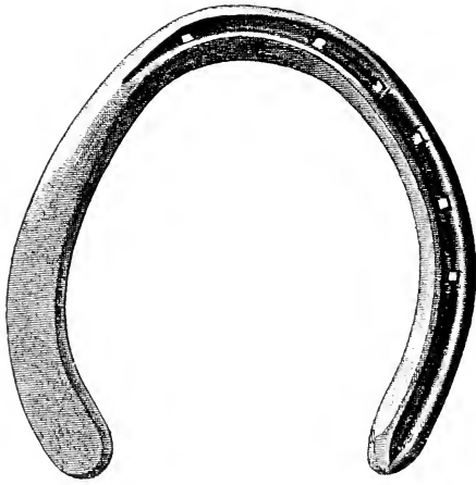
FIG. 298.—Feather-edged fullered concave fore shoe. Made in concave tool from \frac{1}{2} \times \frac{3}{4} inch iron or steel.
