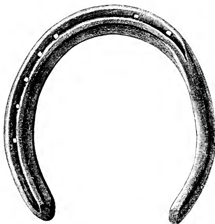
FIG. 294.—Fullered feather-edged concave fore shoe. Made from \frac{5}{8} \times \frac{3}{4} inch iron.
