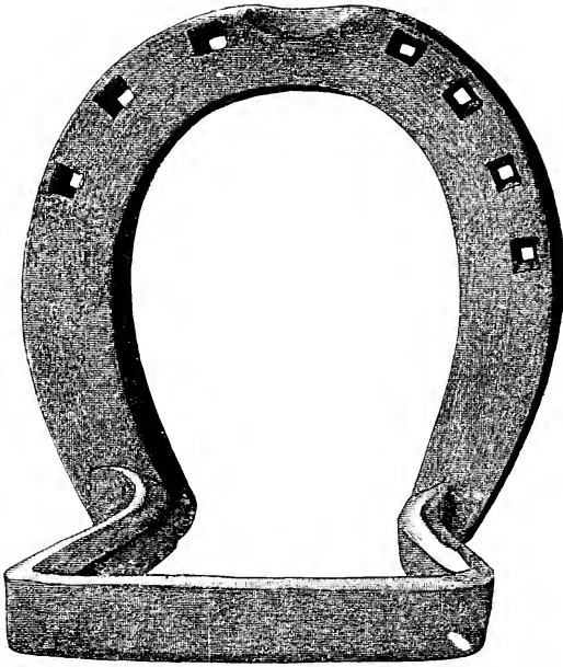
FIG. 393.—Stamped patten fore shoe. Made from \frac{3}{4} \times \frac{1}{2} inch iron.
