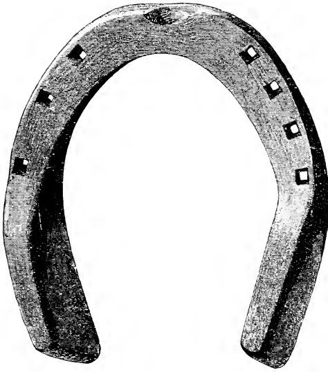
FIG. 389.—Stamped wedge-heeled hind shoe. Made from \frac{3}{4} \times \frac{1}{2} inch iron.
