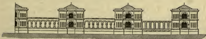
Fig. 8.—Sketch of the end of the southern Pavilions of Herbert Hospital, showing the elevation of the Corridor. (After GALTON.)
