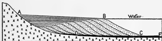
Figure 3 Delta structure: AB topsets; BC foresets; DE bottomsets.
