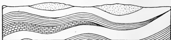
Figure 2 Cross section illustrating pinching or lensing out of strata
