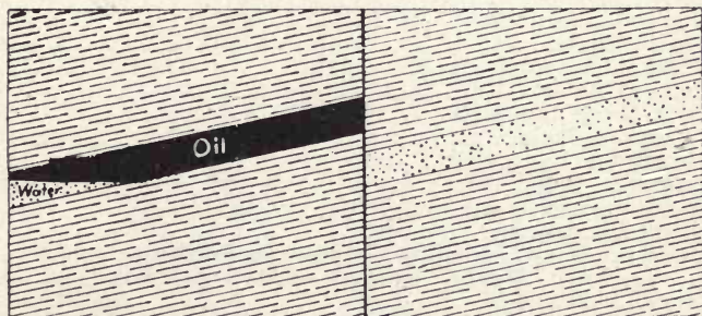
Ideal section showing an oil sand faulted in such a manner that an accumulation of oil will result
