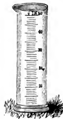
Fig. 68 MEASURE GLASS FOR RAIN GAUGE.
