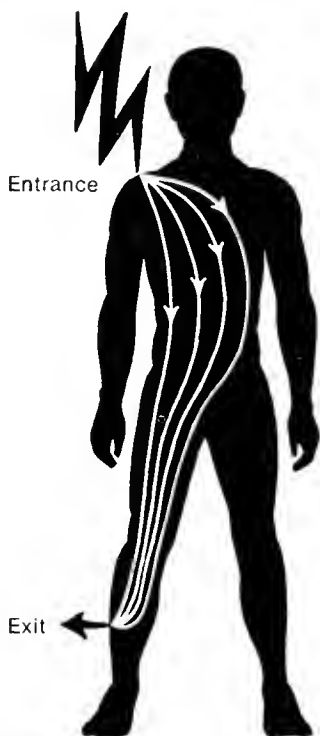
FIGURE 31-3. Path of electrical current in the body. Note spread of current within body. Visible damage will appear only at entrance and exit points.
