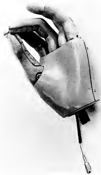
FIGURE 13-5. Northrup-Sierra voluntary opening functional hand without cosmetic cover. Thumb has two possible positions. The thumb position depicted allows for three-finger pinch. The second position, a more open one, allows for grasping of larger objects. Direct external pressure on the thumb controls the position. Using power harnessed from proximal normal joints and muscles, the amputee can voluntarily pull on the cable to move the index and middle fingers together away from the thumb. The ring and little fingers are passive and do not move.
