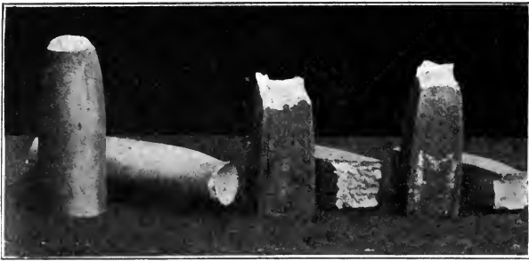
Fractures of Wrought-Iron and Mild Steel in Tension.
