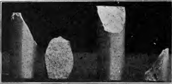
Fractures of Cast-Iron in Compression.
