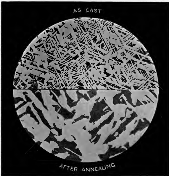
Micrographs of Cast Steel before and after annealing. Magnified 28.5 diameters.
