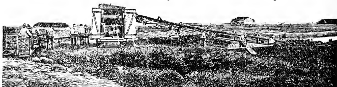
FIG. 162.—Dolberg's peat machine, with conveyer.
