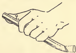
FIG. 15.—Method of holding an engraving chisel.
