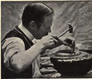
FIG. 3.—Method of holding a chasing tool.
