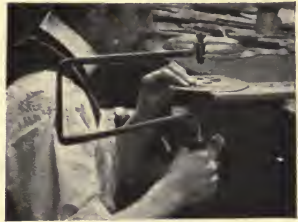
FIG. 7.—Saw piercing in metal.
