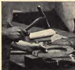
FIG. 2.—Raising a dish on a wood mould.
