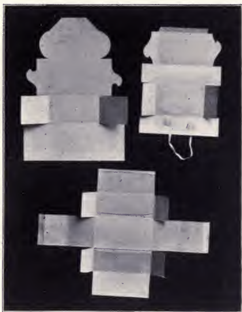
NO. 1 AND NO. 2—ONE-PIECE BOXES. NO. 3.—TWO-PIECE BOX. BOX AND COVER ALIKE.
