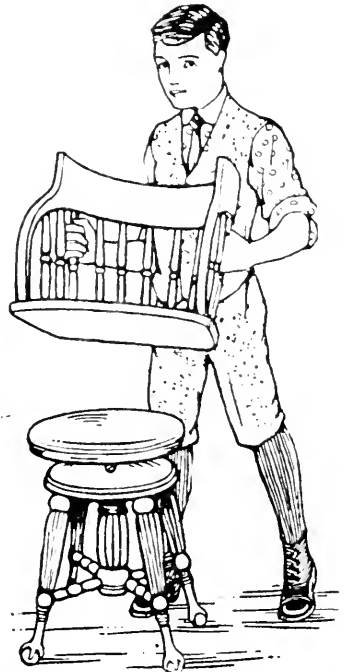
FIG. 190. — How the Seat and Back of a Chair are fastened upon a Piano-stool to form the Office Chair.
