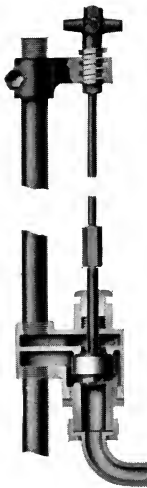
Sectional View of Three Way Valve
