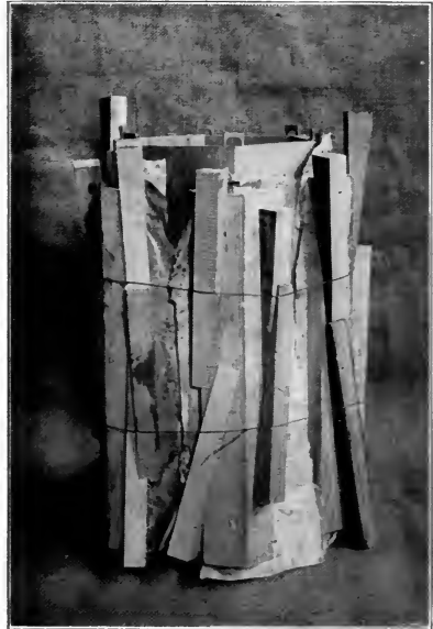
Fig. 256. Gluing up a Column Joint. (Pinch-Dogs at Top of Joints.)
