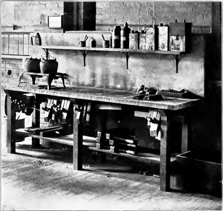
Fig. 243. Gluing and Staining Bench Covered with Zinc.
