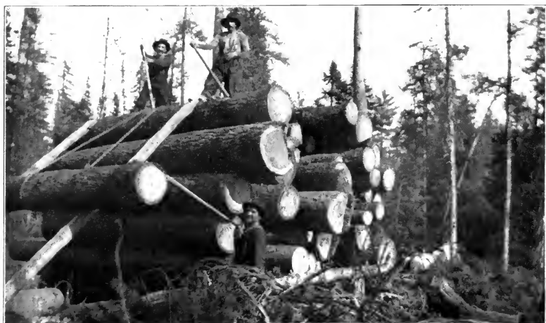
Fig. 11. Decking Logs on Skidway.
