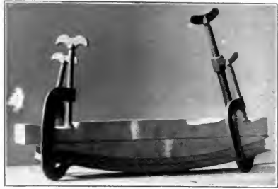
Fig. 299. Bending Boards into Shape after Boiling Them.
