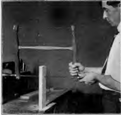
Fig. 95. Using a Turning-Saw.
