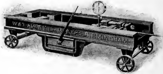
101. MACHINE FOR TESTING ROPES
