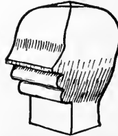
34. STONE BLOCK ROUGHED OUT
