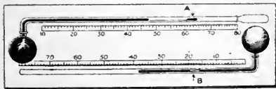
MAXIMUM AND MINIMUM THERMOMETERS A. Maximum Index B. Minimum Index
