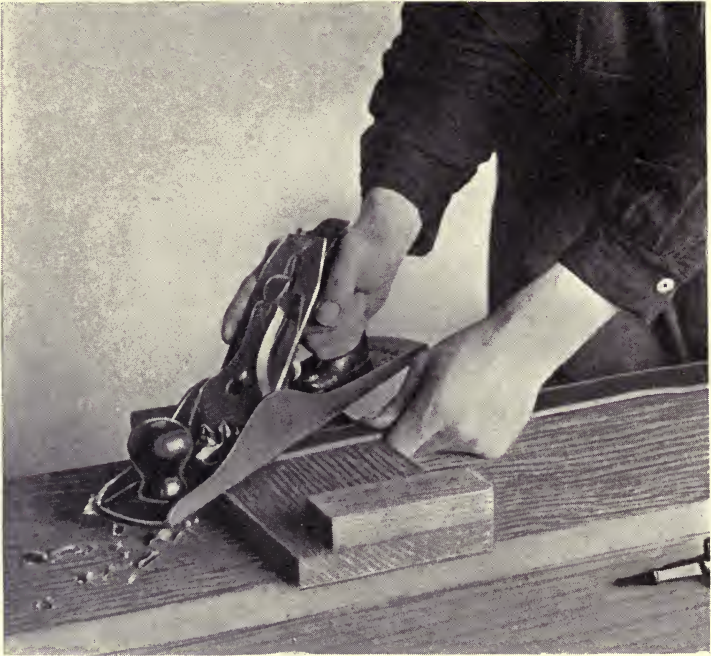
Fig. 12. Skiving the End of the Strap with the Jack Plane.
