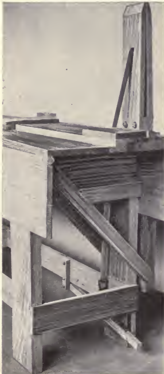
Fig. 29. Lever and Lock of Stitching Clamp and Farm Workbench.
