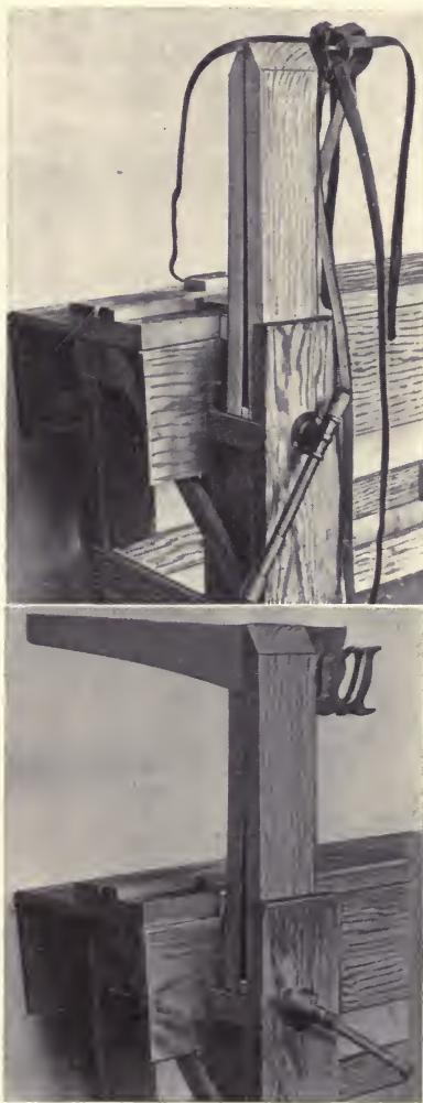
HARNESS STITCHING CLAMP TO BE USED WITH FARM SHOP WORKBENCH VISE
