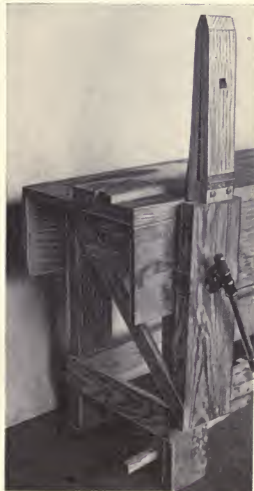
Fig. 30. Stitching Clamp and Vise of Farm Workbench.
