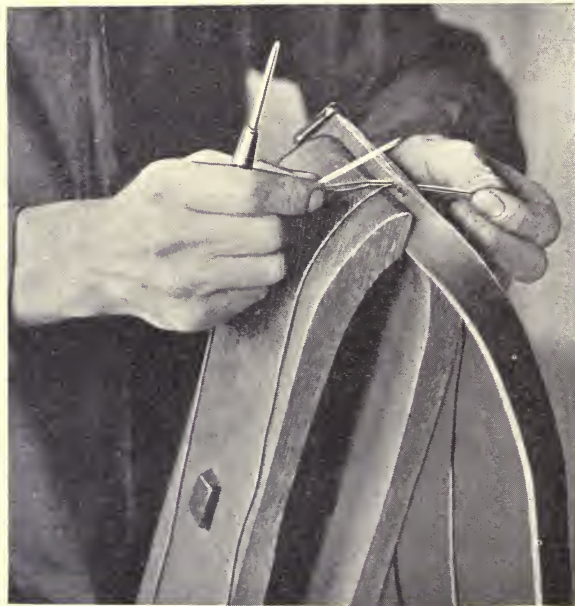
Fig. 14B. Holding Awl and One Needle in Right Hand and Passing the Other Needle Through Hole—View from Side Opposite Workman.
