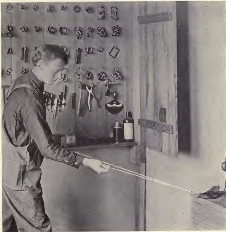
Fig. 8. Equalizing the Wax.
