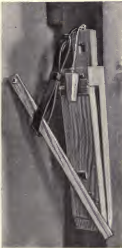
Fig. 32. Clamp, Lever, Wedge and Strap Hung on Nail.
