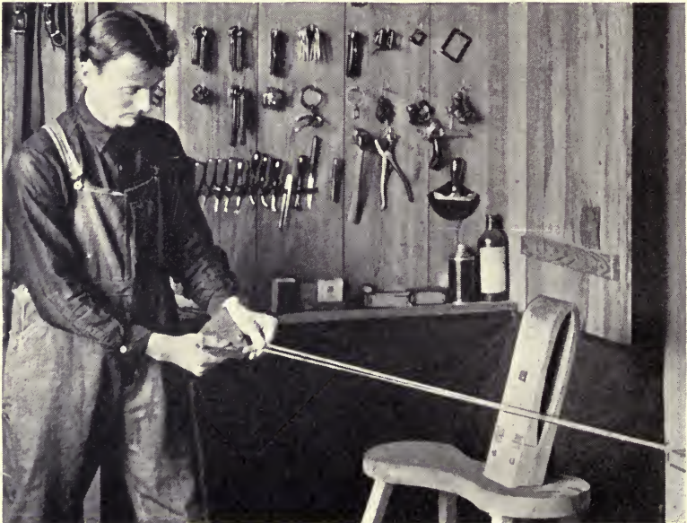
Fig. 4. Waxing the Ends of the Thread.
