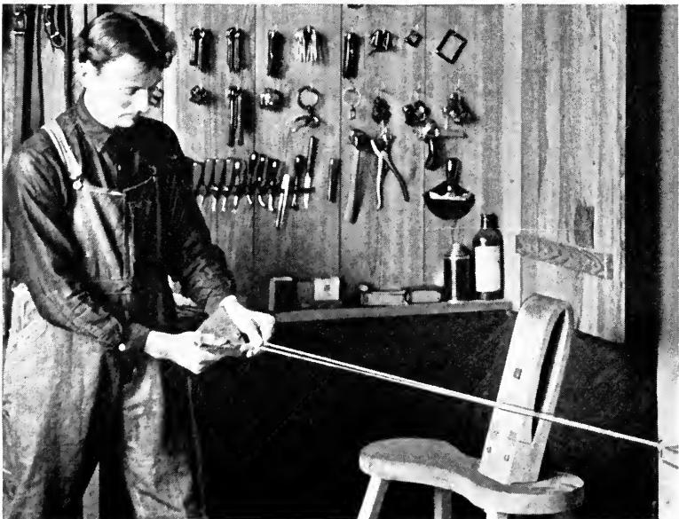
Fig. 4. Waxing the Ends of the Thread.
