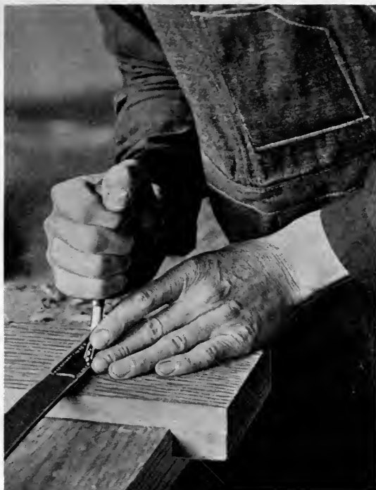
Fig. 15. Finishing the Stitching by Pressing the Wheel Marker over the Stitching.
