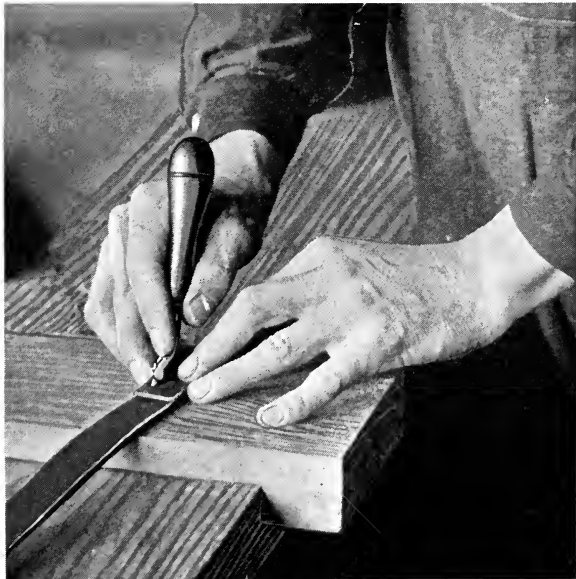
Fig. 13. Spacing Off the Stitching with a Pricking Wheel.
