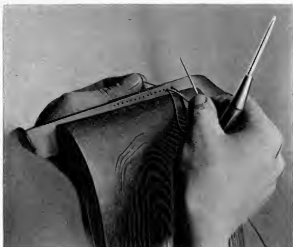
Fig. 14A. Holding Awl and One Needle in Right Hand and Passing Other Needle Through Hole—View from Side of Workman.
