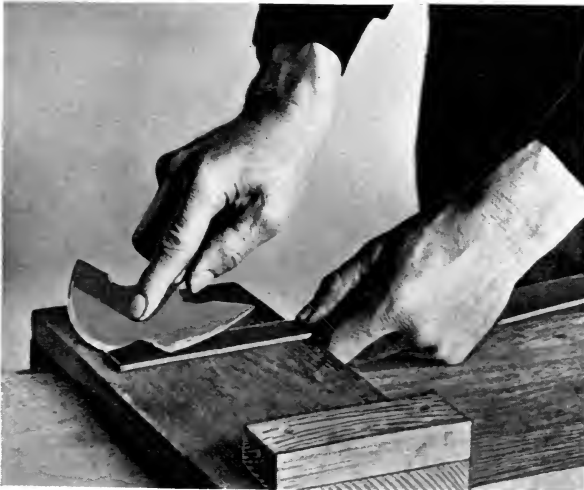
Fig. 11. Skiving the End of the Strap with the Round Knife.
