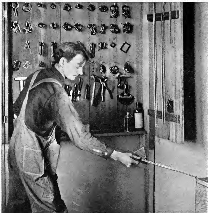
Fig. 7. Waxing the Thread.
