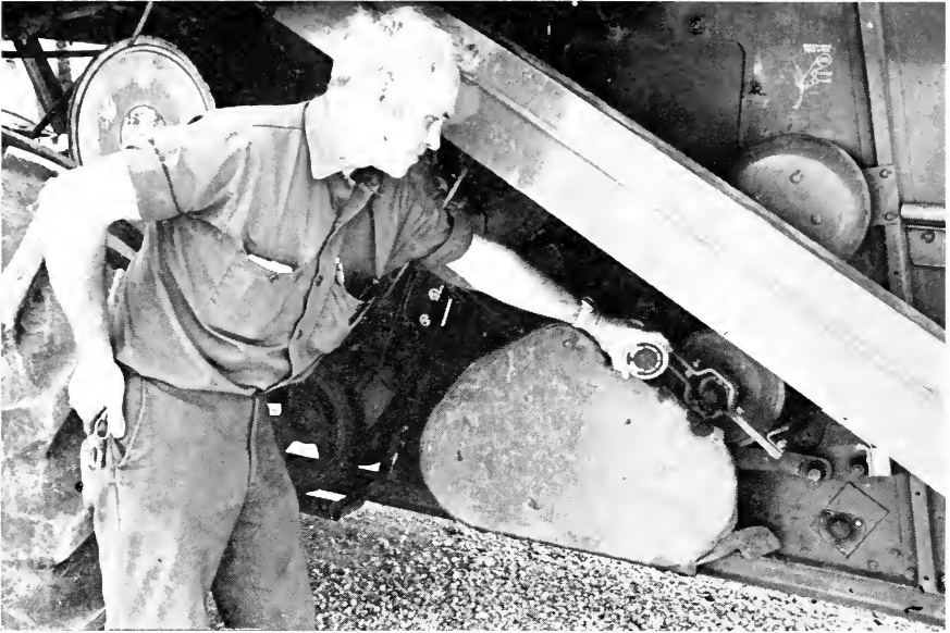
Adjust the fan speed to the crop and feed rate. The air blast from the fan should remove most of the chaff and straw from the soybeans. Adjust the fan for maximum usable air volume without blowing soybeans into the tailings or out the rear of the combine. (Fig. 3)
