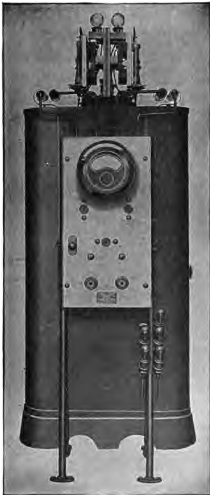
FIG. 2,101.—General Electric 50 light double tube combined unit series mercury arc rectifier outfit; front view. This unit consists of a constant current transformer, reactance, tube tank and exciting transformer mounted on a common base; also a static discharger and pilot lamp mounted on top of the transformer. This arrangement makes the rectifier outfit, with the exception of the switchboard panel, complete in itself.
