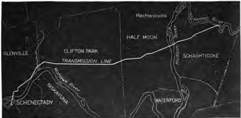
FIG. 2,172. —Course of the Schaghticoke-Schenectady transmission line of the Schenectady Power Co. This transmission line carries practically the entire output of the Schaghticoke power house to Schenectady, N. Y., a distance of approximately 21 miles. The line consists of two separate three phase, 40 cycle, 32,000 volt circuits, each of 6,000 kw. normal capacity. These circuits start from opposite ends of the power house, and, after crossing the Hoosic River, are transferred by means of two terminal towers, fig. 2,173, to a single line of transmission towers. The two circuits are carried on these on opposite ends of the cross arms, the three phases being superimposed. The power house ends of the line are held by six short quadrangular steel lattice work anchor poles with their bases firmly embedded in concrete, the cables being dead ended by General Electric disc strain insulators. This equipment, together with the lightning arrester horn gaps and the heavy line outlet insulators mounted on the roof of the power house, is shown in fig. 2,174. While each circuit carries only 6,000 kw. under normal conditions, either is capable of carrying the entire output of the station; in this case, however, the line losses are necessarily augmented. This feature prevents any interruption of the service from the failure of one of the circuits. There are altogether 197 transmission towers, comprising several distinct types.
