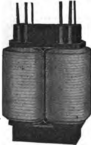
FIG. 1,941.—View showing mechanical construction of coil and core of Moloney pole type \frac{1}{4} to 50 kw. transformer. Moloney standard transformers of these sizes are regularly wound for 1,100 to 2,200 primary volts. For 1,100 volts the primary coils are connected in parallel by means of connecting links; for 2,200 volts, they are connected in series. The porcelain primary terminal board is provided with two connecting links so that connections can be made for either 1,100 or 2,200 volts.
