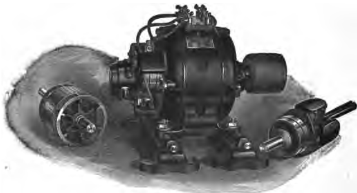
FIG. 1,760. —Holzer Cabot combination polyphase induction motor set, consisting of wound frame and three rotors: 1, squirrel cage armature, 2, wound armature, 3, rotating field. The set is intended for school demonstration of induction motor phenomena. The motor operating with the squirrel cage armature has an inherent constant speed characteristic and on brake tests will show its exceptionally strong starting torque and ability to take excessive overloads. This motor can be used as a generator also, in the sense that if connected to the line and driven above synchronous speed by some external means, it will act as an asynchronous generator and return power to the line. For variable speed service, an armature having a winding upon it similar to that on the frame must be used. External resistances inserted in the armature circuit may be used to produce, first, a reduction of starting current, second, an increase of starting torque, or third, a variation of speed. Thus an extensive list of experiments can be performed with this phase wound armature directly along the line of present engineering practice. The phase wound armature can be used as an alternator in the same sense as mentioned above for the squirrel cage machine. For synchronous motor and three phase operation the revolving field with projecting poles and slip rings would be used, the field being excited from a direct current supply.
