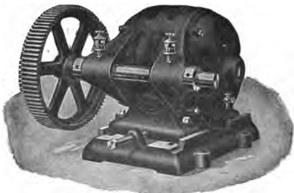
FIG. 1,720.—Triumph back geared polyphase induction motor. A great many applications, especially for direct attachment, require the use of either a very slow or special speed motor. As these are quite costly, the preferable arrangement, and one equally as satisfactory, is the use of a standard speed motor combined with a back geared attachment. Rawhide pinions are furnished whenever possible, insuring smooth running with a minimum of noise.
