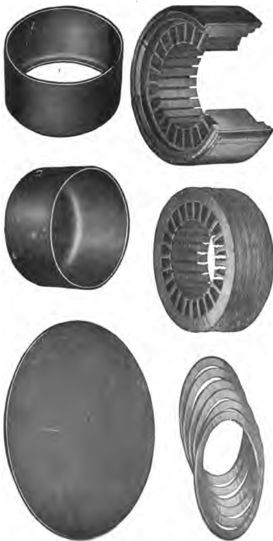
Figs. 1,644 to 1,649. —Construction of General Electric drawn shell fractional horse power motors. The distinguishing feature of drawn shell motors is the field construction which consists of a steel shell or cylinder supporting and clamping together the stator or field punchings. This method avoids the cast frame work outside the active magnetic material. A disc is first punched or "blanked" out of soft steel, fig. 1,644, this disc being faced into the shape, fig. 1,645, with one end closed. The other end of the shell is then cut out, leaving the small flange as in fig. 1,646. It is now ready to receive the core punchings. In the next operation a suitable number of spacing rings, fig. 1,647, are forced into the shell and seated against the retaining lip, which may be seen in fig. 1,646. The field punchings or laminae, fig. 1,648, are now assembled, after which a second and equal set of spacing rings are put into place to center the active field iron. The open edge of the shell is then rolled over the punchings under heavy pressure, thus preparing the field structure for the machinings and fitting of the end heads and base. Fig. 1,649 shows a section of the completely assembled field structure, the parts being cut away to indicate the relation between the field punchings, spacing rings and shell. After the spacing rings at both frame ends have been turned true and grooved, the bearing heads, fig. 1,649, are ready for fastening in place by four fillister headed screws. A complete wound field is shown in fig. 1,858, with flat base casting attached.
