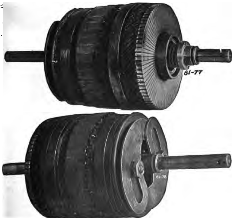
FIGS. 1,874 and 1,875.—Armature of Wagner single phase repulsion-induction commutator motor as seen from the commutator and rear ends, showing the vertical commutator and type of governor employed on the smaller sizes. The operation is explained in fig. 1,873.
