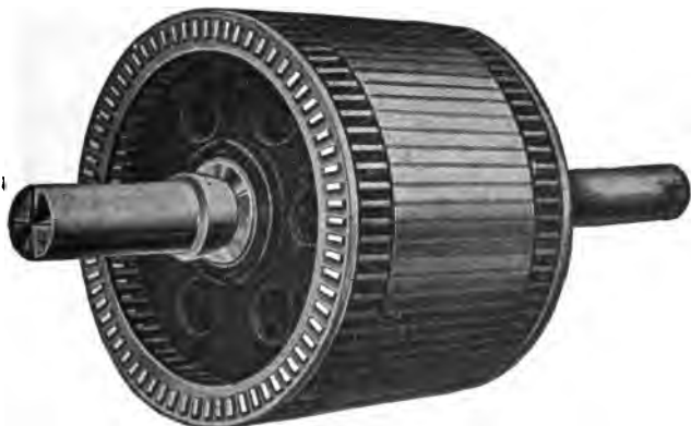
FIG. 1,747.—Triumph squirrel cage armature. In construction thin sheet steel laminations, japanned, are built up to form the core, and are rigidly clamped together by heavy malleable iron end plates. Semi-enclosed slots are punched in the outer periphery to receive the windings, so that none of the centrifugal force is carried by the inductors. These inductors are set edge on, and are riveted and soldered into resistance rings. These rings are punched to receive the inductors in such a manner that there is an unbroken strip of metal completely surrounding them. Moreover, the short circuiting rings are set some distance from the end of the core, so that the inductors between the core and ring act as vanes to force air through the coils for ventilation.
