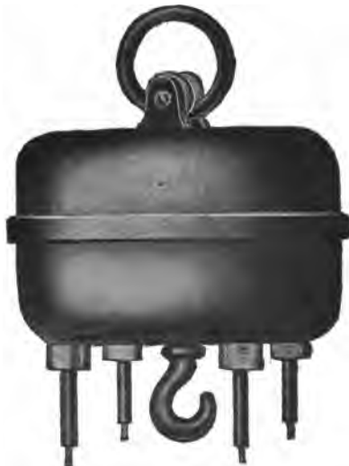
FIG. 2,024.—Moloney flaming auto type arc lamp transformer for 110 volts primary to 55 volts secondary. A hook in bottom of case provides means for suspension of lamp. The transformer may be operated on circuits from 100 to 120 volts primary, 50 to 60 volts secondary. The secondary capacity is 8 to 12 amperes.
