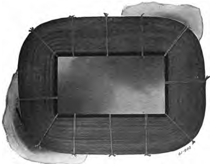
FIG. 1,919. —Wagner transformer coil formed, ready for taping. These are known as "pan cake" coils. They are wound with flat cotton covered copper strip. In heavy coils, several strips in parallel are used per turn in order to facilitate the winding and produce a more compact coil.
