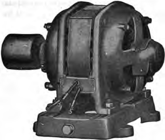
FIG. 1829.—General Electric single phase induction motor. It is suitable for constant speed service where full load torque at starting does not exceed 140 per cent., and in general is adapted to drive all geared and belted machinery requiring constant speed with light or moderate starting torque.
