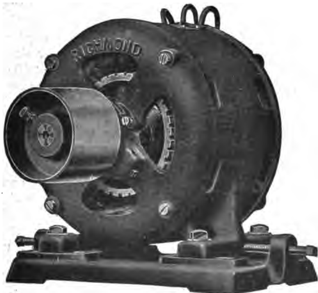
FIG. 1,629.—Richmond three phase induction motor on base fitted with screw adjusting gear for shifting the position of the motor on the base to take up slack of belt.
