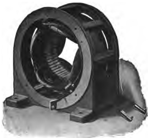
FIG. 1,879. —Field of Sprague single phase compensated repulsion motor. The frame is of the skeleton form which exposes the core, giving effective heat radiation. The single phase field winding is of the distributed concentric type. To facilitate connection to circuits of either 110 or 220 volts, four plainly tagged leads are brought out to the back of the removable terminal board.
