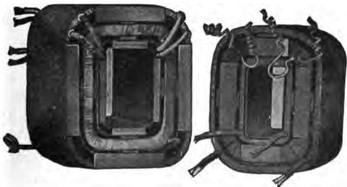
FIGS. 1,921 and 1,922.—Assembled coils of Westinghouse 10 and 15 kva. transformers; views showing ventilating ducts.
