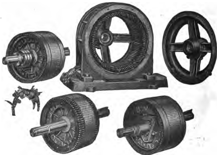
FIGS. 1,773 to 1,778.—Sprague skeleton type motor frame with various types of armature. Fig. 1,777, plain squirrel cage armature; fig. 1,778, internal resistance armature; fig. 1,773, slip ring armature. In the construction of the plain squirrel cage armature, fig. 1,777, copper bars are inserted in the slots of the core, and are insulated from the core by enclosing tubes which project about one-half inch beyond the iron at each side. The bars are short circuited at their ends by copper rings. These rings are thin, but of considerable radial depth and are held apart by spacing washers. They have rectangular holes punched near their outward periphery, through which the armature bars pass, and to which they are soldered. The internal resistance armature, fig. 1,778, is provided with a phase winding, starting (internal) resistance, and switch located on the shaft. The starting resistance is designed to give approximately full load torque with full load current at starting. A greater torque than full load torque can be obtained for starting, if required, by cutting out resistance. The resistance consists of cast iron grids enclosed in a triangular cover which is bolted to the end plates holding the armature laminæ together, and is short circuited by sliding laminated spring metal brushes along the inside surface of the grids. The brushes are supported by a metal sleeve sliding on the shaft which is operated by a lever secured to the bearing bracket and located just above the bearing. A rod passing through the end of the shaft operates the short circuiting arrangement in sizes up to about 25 horse power. The external resistance or slip ring armature, fig. 1,773, is similar in construction to fig. 1,778, with the exception that slip rings are provided because of the external location of the resistance. These rings connect the inductor through brushes to a controlling and external resistance, two or more carbon brushes being provided for each ring, as in fig. 1,776.
