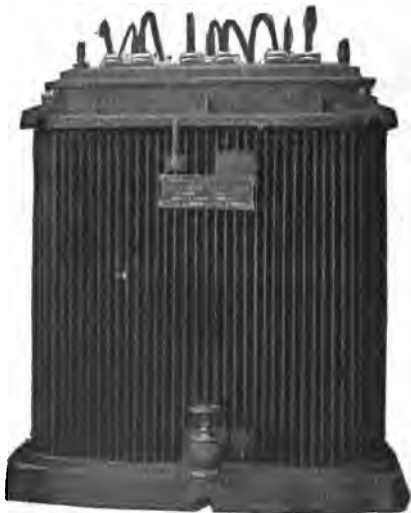
FIG. 1,968. —Wagner 300 kva, 4,400 volt three phase oil cooled transformer. In this type of transformer the case is filled with oil and fluted so as to increase the cooling surface, an oil drain valve is screwed to a wrought iron nipple cast into the base, the duct to which is in such a position as to make it possible not only to drain all of the oil from the transformer, but when desirable, to draw off a small quantity from the bottom. Should any moisture be in the oil it is therefore drawn off first.
