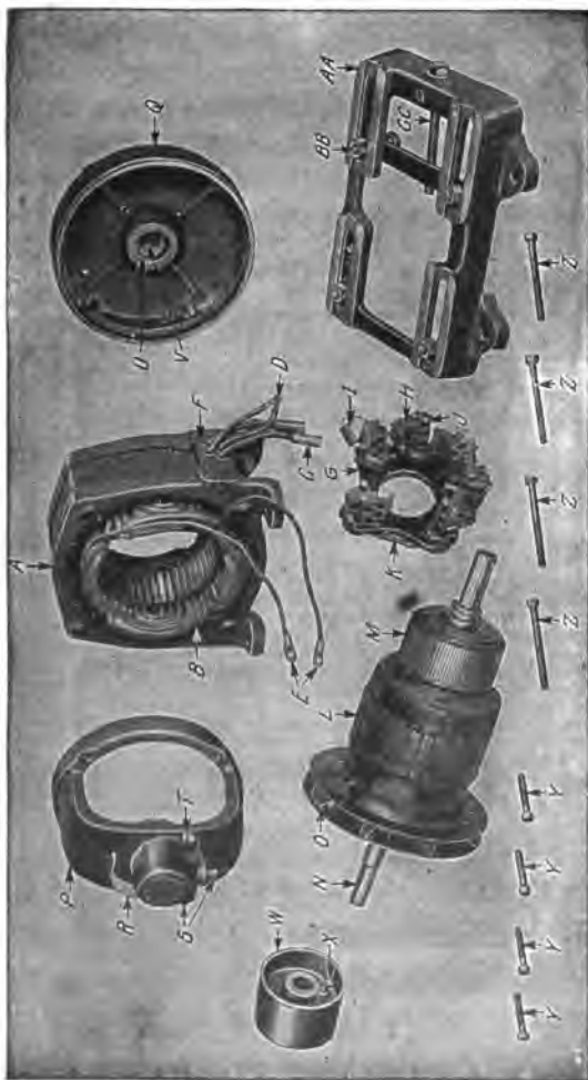
FIG. 1,894 to 1,908. —Parts of General Electric single phase compensated repulsion motor. The field frame employs the riveted form of construction, so that the ends of the laminations are exposed directly to the air, insuring low operating temperatures and high overload capacity. The field winding consists of a main winding of the distributed concentric type, and a compensating winding. The series type of winding is employed, and the completed rotor is treated with a special insulating compound, which renders the coils moisture proof under ordinary conditions. On motors of more than 2 horse power capacity a ventilating fan is attached to the rotor which provides a continuous supply of cool air while the motor is in operation. Two types of brush holder yoke are used. The smaller motors use a moulded yoke of insulating compound, reinforced by a cast iron L section ring embedded in the moulded structure. Cast iron yokes are used on larger motors. The brushes are of carbon with copper pigtails which carry all the current. The brushes in this machine remain permanently in contact with the commutator. The parts are: A, field; B, field winding; C, line terminal; D, tube terminal; E, compensating terminal; F, terminal board; G, brush yoke; H, brush holder; I, carbon brush; J, brush stud; K, short circuit connection; L, armature; M, commutator; N, shaft; O, fan; P, commutator end shield; Q, pulley end shield; R, oil well cover; S, oil gauge; T, oil gauge; U, bearing lining; V, oil ring; W, pulley; X, pulley set screw; Y, commutator end shield holding bolts; Z, pulley end shield holding bolts; AA, base; BB, float bolts; CC, belt tightener screw.
