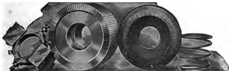
Figs. 1,880 to 1,884. —Assembly and disassembled view of short circuiting device as used on Bell single phase repulsion induction motor. The armature, which is wound in a similar manner to those used in direct current motors, has a commutator, and brushes, which being short circuited on themselves, allow great starting torque, with small starting current. The motor starts by the repulsion principle, and on reaching nearly full speed, a centrifugal governor pushes the copper ring against the commutator segments, thereby short circuiting them, and the motor then operates on the induction principle.
