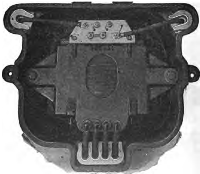
FIG. 1965.—Looking down into a Wagner central station transformer, showing the connection board, which provides facility for varying the ratio of transformation and also for interchanging the primaries.
