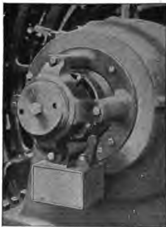
FIG. 2,062.—Mechanical oscillator and speed limit device of Westinghouse commutating pole rotary converter. It automatically prevents the armature of the converter remaining in one position and thus not allowing brushes to wear grooves in both commutator and collector rings. The oscillator is a self-contained device carried at one end of the shaft. The operating parts consist of a hardened steel ball and a steel plate with a circular ball race, backed by a spring. The machine is so installed with a slight inclination toward the end carrying the oscillator. As the armature revolves the ball is carried upward and owing to the convergence of the steel race and shaft face, the spring is compressed. The reaction of the spring forces the armature away from its natural position and allows the ball to drop back to the lowest point of the race.
