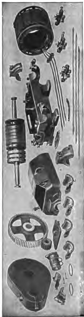
Figs. 1,801 to 1,828. —Disassembled view of Western Electric three phase external resistance or slip ring mill type induction motor. It is adapted to severe working conditions, such as are met with in steel mills, crane and hoist service, etc. Designed for 220 or 440 volt, 25 cycle circuits. The frame is divided horizontally into an upper and a lower steel casting, both of which are bolted together at the corners by four heavy bolts. The lower casting is provided with four feet for bolting the motor to its foundation. The end of the upper frame which covers the slip rings is equipped with malleable iron covers held in place by lock bolts. The field and armature are of the usual construction. One end of the armature winding is protected against mechanical injury by the slip rings which are of heavy construction and of practically the same diameter as the armature, and the other end by a detachable flange of the same diameter as the outside of the winding. The slip rings are mounted on the same spider as the armature, so that the shaft can be removed without disturbing any of the connections. The brushes are equipped with riveted pigtails, and held in brass brush boxes machined to gauge. Heavy coiled clock springs are used to maintain an even pressure of the brushes on the slip rings. The armature leads are brought out through holes in the upper half of the frame, and the field leads are brought through a block, which fits in an opening in the upper edge of the lower half.
