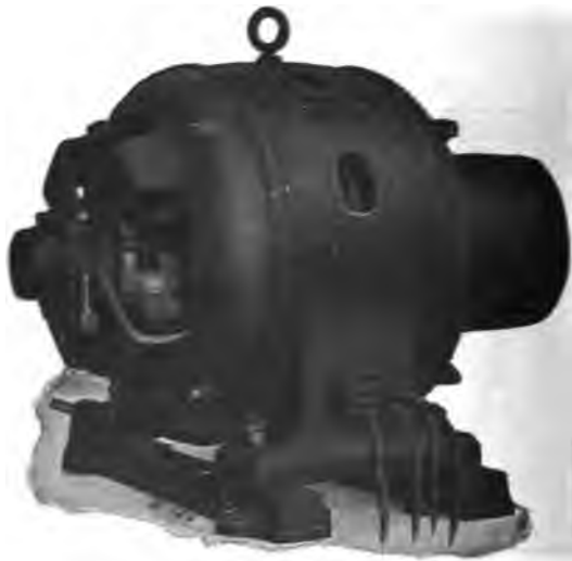
FIG. 1,873.—Wagner single phase repulsion induction commutator motor. Its working principle is repulsion start and induction operation . Starting with the machine at rest, brushes in pairs cross connected through a low resistance conductor, bear upon the commutator, temporarily short circuiting the armature winding then developing a strong starting torque on the repulsion principle. On attaining full load speed the individual segments of the commutator are all positively connected together by the operation of an automatic centrifugal governor, thereby transforming the armature winding to the squirrel cage form, the motor then continuing as an induction motor. The governor at the same time removes the brushes from contact with the commutator to save wear. If the power service should fail for any reason, the motor returns to the starting condition, and picks up its load when the power comes on again without attention of the operator.
