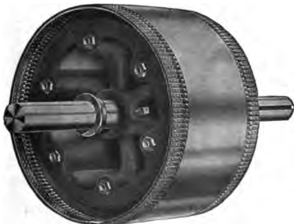
FIG. 1,757.—Richmond squirrel cage armature. The copper bars are double riveted at either end to the resistance rings, then dipped into a solder bath.
