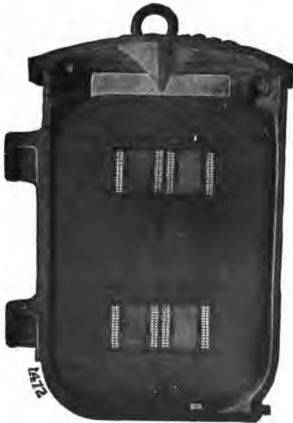
FIG. 1,969. —Section through Fort Wayne (type A) transformer showing interior of case, core conductors, and insulation, also division of laminæ.
