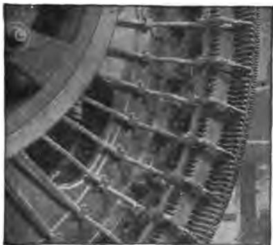
FIG. 2,044. —Equalizer connections of Westinghouse rotary converter. The armature coils are cross connected at points of equal voltage and taps are led out from the winding at suitable points to the slip rings. This construction insures a uniform armature saturation below each pole piece and eliminates one cause of sparking at the commutator.
