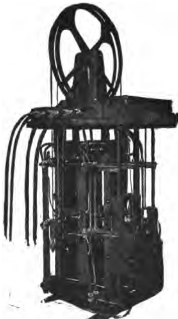
FIG. 2,092.—75 light Westinghouse-Cooper Hewitt mercury vapor rectifier constant current regulating transformer with case removed. The transformer is of the repulsion coil type, oil cooled and oil insulated. It is so arranged as to give a constant secondary current and to insulate the arc lines from the primary circuit. The regulating transformer contains two stationary secondary coils and two moving primary coils balanced against each other. Each secondary coil of the 75 light regulator is wound in two parts, owing to the use of two rectifier bulbs in series in outfits of this capacity. The repulsion between the primary and secondary coils changes the distance between them according to the variation of load, and the induced current in the secondary is thus kept constant. An increase in current causes the primary and secondary coils to separate, and a decrease in current permits them to approach each other, until the normal balance is restored. The moving coils are hung from sheave wheels having roller bearings and are balanced so that they are sensitive to the slightest impulse tending to separate them or draw them closer together. (See figs. 1,981-2, and 2,111.) The windings are insulated for a voltage considerably in excess of that existing in normal service. Several taps are provided to take care of different voltages and wave forms. A combination of taps will be found which will be suitable for any wave form coming within the American Institute of Electrical Engineer's limits for a sine wave. The secondary coils are also provided with taps for 85 per cent. of normal load, so that less than normal load can be taken care of at a good power factor. Any part of the full load can be carried temporarily with the full load connections of the transformer, but at permanent light loads the power factor and efficiency will be improved by using the 85 per cent. connections. Standard regulating transformers are wound for 6.6 and 4 amperes, and for primary circuits of 220, 440, 1,100, 2,200, 6,600 and 13,200 volts. Regulators can be specially wound for 5.5 amperes. For three phase circuits three regulators can be used, one on each phase, or they can be furnished in pairs with an auxiliary auto-transformer to give a balanced load. The regulators can be connected, in cases where the unbalancing is not objectionable, to separate phases.
