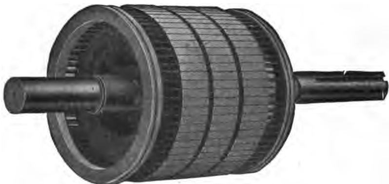
FIG. 1,752. —Fairbanks-Morse squirrel cage armature with cast-on rings showing inspection grooves. The method consists in fusing the ends of the inductors into an end ring of a special composition, thereby producing a perfect electrical and mechanically strong joint. In this process the armature with its bars in place is put into a mould and the molten metal poured around the inductors, melting their ends and effectually fusing them into the body of the ring. The ring is then turned down to finished size and polished. An inspection groove is cut as shown to indicate that the fusion is complete and the joint perfect.
