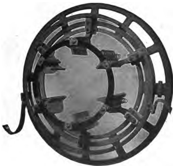
FIG. 2,047.—Westinghouse rotary converter brush rigging showing method of bracing the brushes. The brushes are supported by a rigid cast iron rocker ring which fits accurately in the frame. A handwheel worm and screw arrangement for shifting the brushes is provided. Cast iron arms bolted to, but insulated from the rings, carry the rods on which the brush holders are mounted. Brush holders are of brass cast in one piece, of the sliding type and have braided copper shunts. Brush tension is adjustable.
