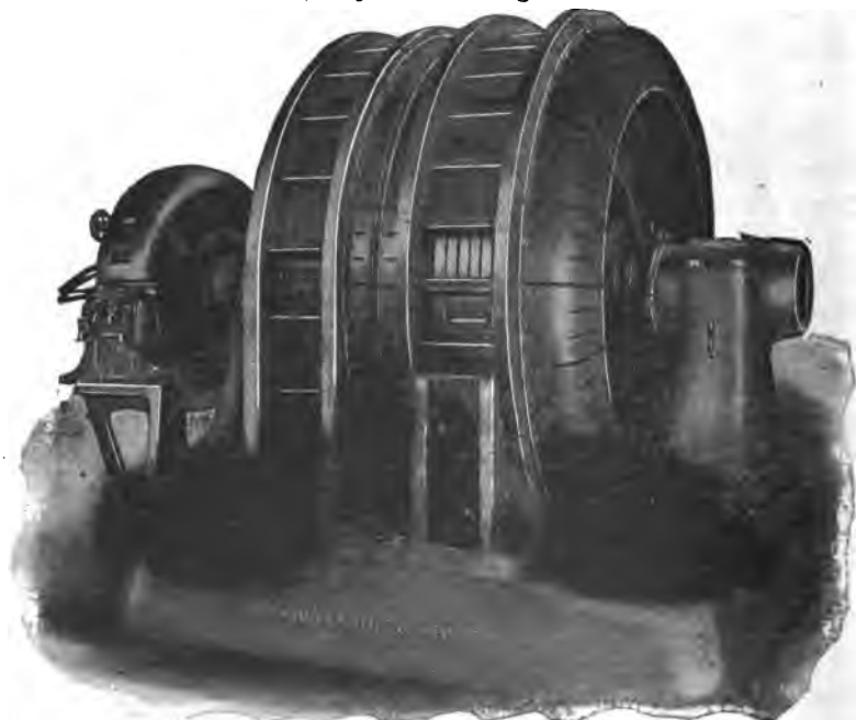
FIG. 2,069.—General Electric frequency changer set, consisting of a 11,000 volt synchronous motor with direct connected exciter and a 2,300 volt alternator.
