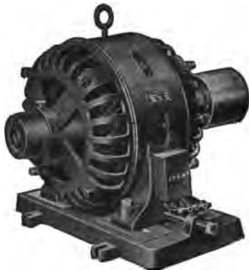
FIG. 1,650. —Ideal fifteen horse power two phase induction motor. The armature core is supported by a cast iron frame carried on a base, with sliding ways and screw adjustment for tightening the belt. The armature core is provided with ventilating apertures, with metal spacers between each tooth. The revolving field is a steel casting with radially projecting poles, to which the pole shoes are bolted. The overhanging pole tips retain the field coils. All coils of the smaller sizes are wound with insulated copper wire of square section, and of the larger sizes, with flat copper, wound on edge, each turn being insulated by sheet insulation. Motors of this type are adapted for use in small power plants and isolated plants. The relatively high speed for which they are designed, reduces considerably the weight and overall dimensions, and likewise the cost. The exciter is belt driven. The normal kw. capacity of the exciter usually exceeds the kw. required for the excitation under normal load conditions to permit of station lighting. All exciters are built as compound wound dynamos, capable of delivering the exciter current up to 125 volts, which is sufficient margin in the field to control the alternating current line voltage on circuits of unusually low power factor.
