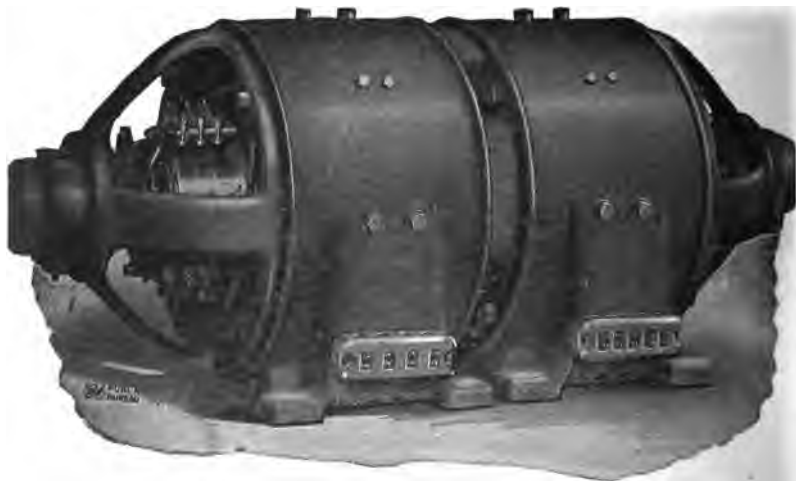
FIG. 2,073. —General Electric 9.5 kw. 1,000 R.P.M. balancer set. This is a form of direct current compensator, the units of which it is composed may be alternately motor or generator, and the secondary circuit is interconnected with the primary. Balancer sets are widely used to provide the neutral of Edison three wire lighting systems. They are also installed for power service in connection with the use of 250 volt motors on a 500 volt service or 125 volt motors on a 250 volt service. Although the balancer set may be manufactured for more than one intermediate voltage, the General Electric Company recommends the three wire system as it is simpler. The motors may be more equally divided and the reserve margin of the motor is more conservative for that class of work requiring increase in torque with decrease in speed. The voltage of the system being given, the capacity of a three wire balancer set is fixed by the maximum current the neutral wire is required to carry. This figure is a more definite specification of capacity than a statement in per cent. of unbalanced load. As designed for power work and generally for lighting service, the brushes of each machine are set at the neutral point in order to get the best results for operating alternately either as a generator or motor. Where the changes of balance are so gradual as to permit of hand adjustment if desired, a considerable increase in output is obtainable.
