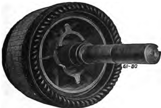
FIG. 1,763. —View of armature interior of Wagner polyphase induction motor with wound armature, showing the centrifugal device which at the proper speed short circuits all the coils, transforming the motor to the squirrel cage type. The winding is connected with a vertical "commutator" so called. Inside the armature are two governor weights, which are thrown outwards by the centrifugal force when the machine reaches the proper speed, thus pushing a solid copper ring (which encircles the shaft) into contact with the inner ends of the "commutator" bars, thus completely short circuiting the armature winding.
