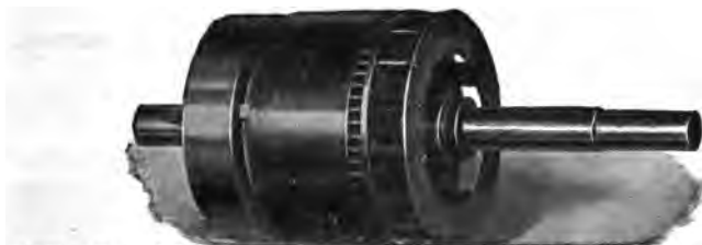
FIG. 1,851.—General Electric high resistance clutch type smooth core squirrel cage armature of single phase induction motor. The core laminæ are slotted near the circumference to retain the bar inductors, which extend beyond the core at either end where they are permanently connected to heavy short circuiting rings.
