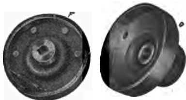
FIGS. 1,856 and 1,857.—Partly assembled clutch pulley. F, internal mechanism comprising parts A, B, C, of fig. 1,852. G, outer shell and pulley, comprising parts D and E of fig. 1,852.
