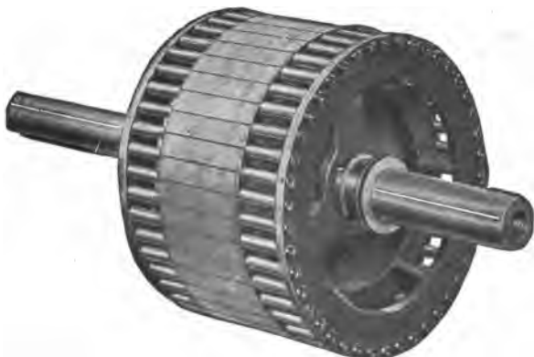
FIG. 1,746.—Allis-Chalmers squirrel cage armature construction. The core laminae are mounted on a cast iron spider having arms shaped to act as fan blades for forcing air through the motor. The spider is pressed on to the shaft. In the smallest sizes the punchings are mounted directly on the shaft, which is properly machined to hold them firmly. Copper bars are used as inductors in the larger sizes, and copper rods in the smaller sizes. The ends of the inductors are turned down somewhat smaller than the body and fit in holes in the end rings. The shoulder thus formed fits firmly against the end rings. Good electrical contact is obtained by expanding the inductors in the end ring holes. In large armatures both bars and end rings are of rectangular cross section, the bars and rings being fastened by machine steel cap screws.
