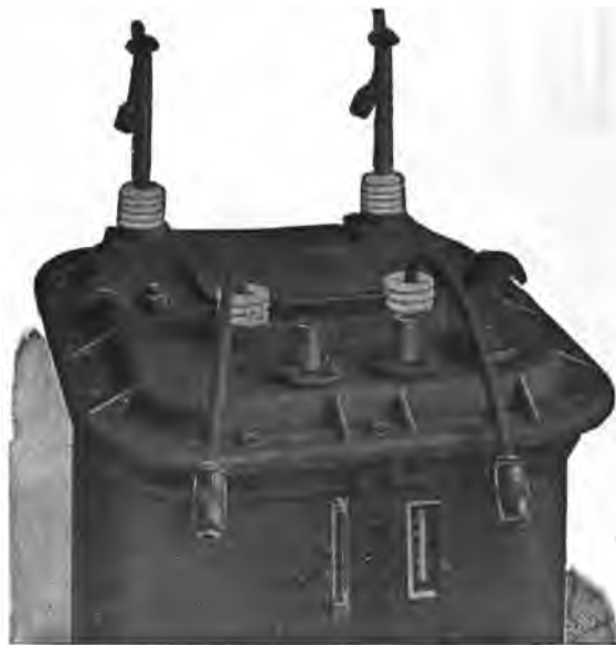
FIG. 1,945. —Cover construction of Wagner 350 kva., oil filled 1,100-2,200 volt transformer. In transformers with corrugated cases, the base and top ring are cast to the corrugated iron sheets.
