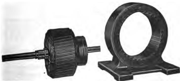
FIGS. 1,865 and 1,866.—Fort Wayne split phase fractional horse power induction motor with stationary armature. The object of placing the squirrel cage armature winding on the stationary part or frame is to decrease the radial depth of the latter more than would be possible with the usual arrangement where the armature forms the rotating part. The small radial depth of the stationary armature makes possible a revolving field of maximum diameter giving in turn an exceptionally large air gap area, which reduces the magnetising current, hence improves the power factor of the motor.
