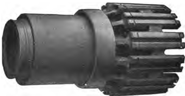
FIG. 2,043. —Westinghouse rotary converter armature spider. It is made of cast iron or cast steel. The dovetail grooves are machined in the feet or ends of the arms and in these slots the laminations forming the armature coil engage.
