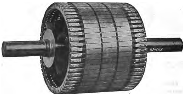
FIG. 1,756. —Wagner squirrel cage armature for polyphase induction motor, as employed on motors of from 5 to 25 horse power. The features of construction as seen in the illustration are bar inductors, ventilating passages through the core laminae, riveted connection between inductors and end rings ventilating vanes on end plate, extra large end rings. The object of making the rings unusually large is to make the resistance of the rings lower than is desirable for some classes of service, in order to obtain motors having minimum slip, increased efficiency, and maximum overload capacity under normal operation. When the torque required by some very unusual and entirely abnormal installation exceeds that of the average conditions, it is an easy matter to reduce the section of the end rings, by turning them down in a lathe, thereby increasing the resistance and starting torque.
