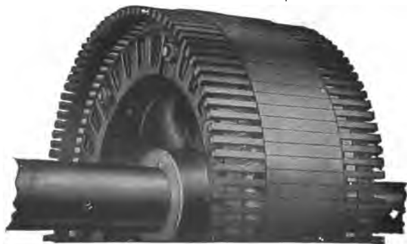
FIG. 1,749. —General Electric welded form of end ring construction on squirrel cage armatures. Space limitations make it difficult to provide multiple soldered rings of sufficient area for large motors; hence, on such machines welding is resorted to, as shown. The ring in welded construction is placed beneath the bars at each end of the armature. Short radial bars are welded to the edges of these rings and to the inductors or squirrel cage bars, thereby making good electrical contact.
