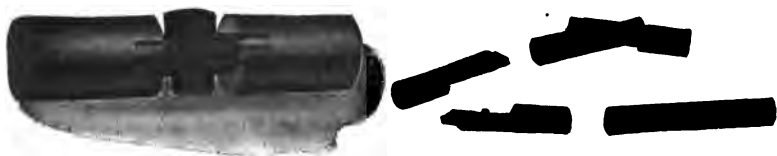
FIGS. 1,949 to 1,953.—Westinghouse low tension transformer connectors for connecting the low tension leads to the feeder wires. The transformers of the smaller capacities have knuckle joint connectors and those of the larger sizes have interleaved connectors. These connectors form a mechanically strong joint of high current carrying capacity. Since the high tension leads are connected directly to the cut out or fuse blocks, connectors are not required on these leads. The use of these connectors allows a transformer to be removed and another of the same or a different capacity substituted usually without soldering or unsoldering a joint. The connectors also facilitate changes in the low tension connections.
