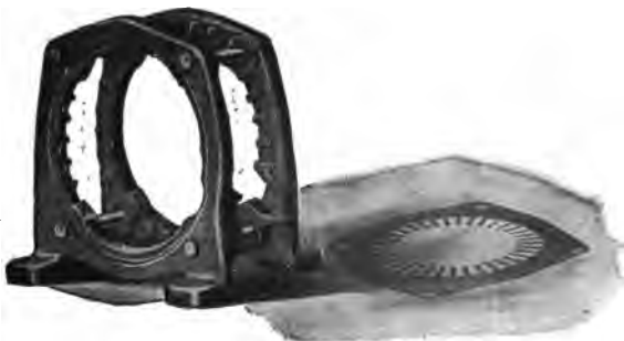
FIGS. 1642 and 1643. —Western Electric end flange rivets and punchings of riveted frame induction motor. The riveted frame is constructed of two cast iron flanges between which the stator laminations of sheet steel are securely clamped and riveted under hydraulic pressure. This construction exposes the laminations directly to the air and improves the radiation, thus insuring high overload capacity and low operating temperatures. The field slots are overhung or partially closed, affording mechanical protection to the coils.
