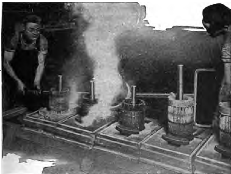
FIG. 1,915.—Method of casting end rings on squirrel cage armatures of Fairbanks-Morse induction motors. The metal being fused to the bars at a temperature in excess of 1,832 degrees Fahr. it is readily seen that the destructive effect of any subsequent heating is eliminated. While giving the most intimate contact at the joints, a multiplicity of joints is avoided as well as solder.
