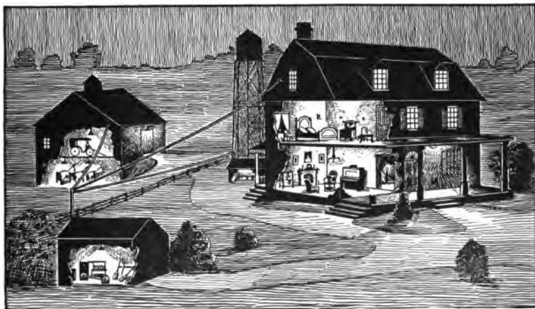
FIG. 2,145. —View of a typical isolated plant. The illustration represents an electric lighting plant on a farm showing the lighting of the dwelling, barn, tool house and pump house. The installation consists of a low voltage dynamo with gas engine drive and storage battery together with the necessary auxiliary apparatus.
