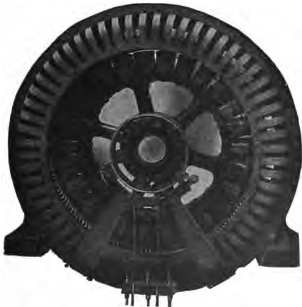
FIG. 1,810. —Westinghouse self-starting synchronous motor. Motors of this type are suitable for constant speed service where starting conditions are moderate, such as driving compressors, pumps, and large blowers. Synchronous motors can be made to operate not only as motors but as synchronous condensers to improve the power factor of the circuit. The field is provided with a combined starting and damper or amortisseur winding so proportioned that the necessary starting torque is developed by the minimum current consistent with satisfactory synchronous running without hunting. The armature slots are open and the coils form wound, impregnated, and interchangeable. Malleable iron finger plates at each end of the core support the teeth. Ventilating finger plates assembled with the laminations form air ducts. The frames are of cast iron, box section with openings for ventilation; shoes and slide rails permit adjustment of position. The brush holders are of the standard sliding shunt type. Two or more brushes are provided for each ring.
