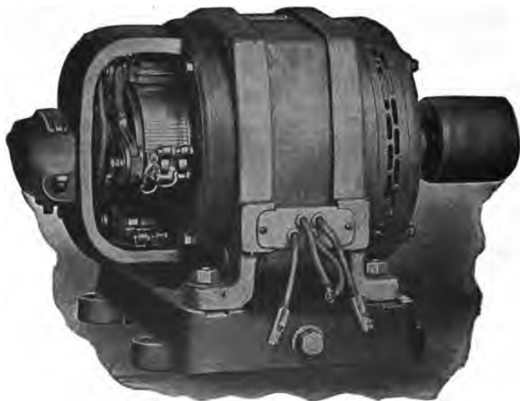
FIG. 1,876.—General Electric single phase compensated repulsion motor. The frame is of the riveted form and the field winding consists of distributed concentric coils, each being separately insulated and taped up to each core slot. The compensating winding (depending usually on the size of frame), forms either the center portion of the main winding or a separate winding concentric therewith. The polar groupings are arranged for a frequency of 25 and 60. There are four terminal leads permitting interchangeability of operation on 110 or 220 volt circuits. By connecting adjacent pairs of these terminals in multiple, motors of this type are made adaptable for 110 volt service; for double this pressure the four leading in wires are connected in series. The motor will operate satisfactorily where the arithmetical sum of voltage and frequency variation does not exceed 10 per cent.; that is, the voltage may be 10 per cent. high if the frequency remain at normal, or the frequency may be 10 per cent. high assuming no variation in voltage. A decrease of 5 per cent. in frequency accompanied by a similar increase in voltage is permissible or, as above stated, any similar combination whose arithmetical sum is within 10 per cent. of normal. The armature winding is of the series drum type connected to a commutator carrying two sets of brushes, each set being displaced electrically from the other by 90 degrees. The first set, known as the energy brushes , is permanently short circuited and disposed at an angle to the lines of field or primary magnetization, as in an ordinary repulsion motor. The second set, or compensating brushes , is connected to a small portion of the primary winding included in the field circuit, so as to impress upon the armature an electromotive force, which serves both to raise the power factor and at the same time maintain approximately synchronous speed at all loads. The armature laminations are built up on a cast iron sleeve having the same inside bore as the commutator. In case the shaft become damaged or worn, it can be readily pressed out and replaced without disturbing the commutator or windings. The motor is connected to run counter clockwise. Clockwise rotation is obtained by interchanging the leads to the compensating brushes and slightly shifting the brush holder yoke. This type motor may be thrown on the line without the use of a rheostat, and is suitable for operating refrigerating machines, air compressors, house pumps or similar apparatus where a float switch or pressure regulator is used to close or open the supply circuit.
