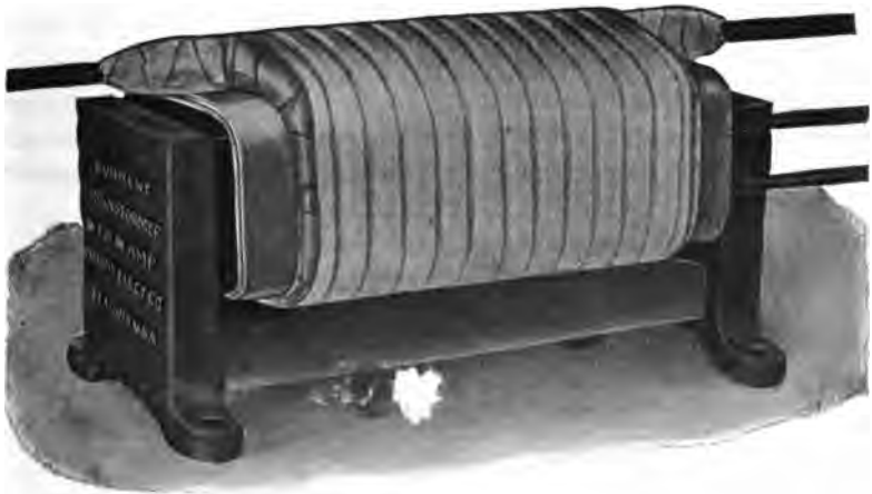
FIG. 2,018. —Moloney current transformer switchboard or indoor type. It is used ordinarily for insulating an ammeter, a current relay, the current coil of a watt meter or watt hour meter from a high tension circuit, for reducing the line current to a value suitable for these instruments.
