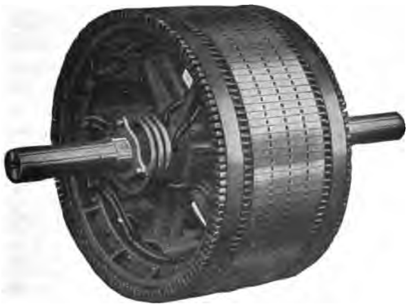
FIG. 1,800.—Allis-Chalmers phase wound external resistance type or slip ring armature construction. The winding is for three phases and the terminals are brought out to three slip rings. The front bracket is slightly modified to make room for these rings on the inside. For starting duty sufficient resistance is supplied to reduce the starting current taken by the motor to 1\frac{1}{4} times the normal full load current. In the running position the resistance is all cut out of the circuit. For speed regulation sufficient resistance is supplied to reduce the speed 50% on normal full load torque.
