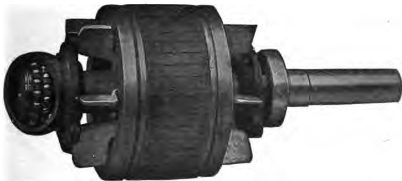
FIG. 1,913.—Fairbanks-Morse squirrel cage armature, showing ball bearings.
