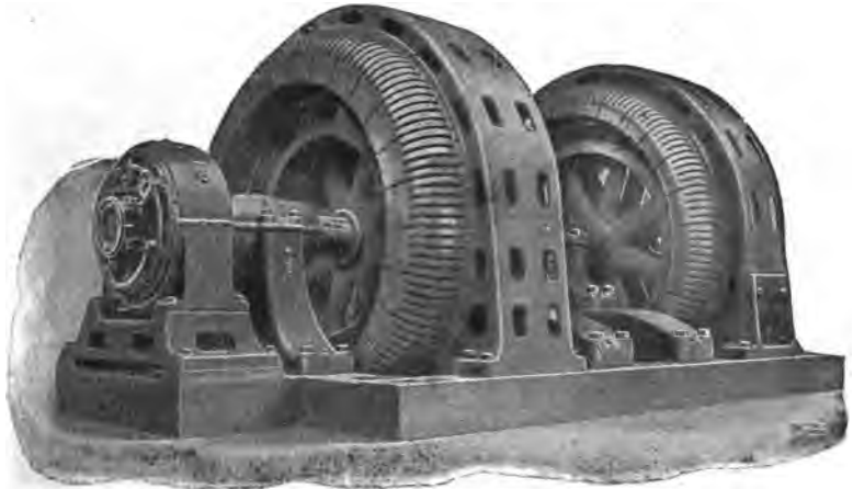
FIG. 2,070.—General Electric four unit frequency changer set consisting of a 11,000 volt synchronous motor, 13,200 volt alternator, 250 volt exciter, and 440 volt starting induction motor. Where parallel operation is required between synchronous motor driven frequency changers, a mechanical adjustment is necessary between the fields or armatures of the alternator and motor to obtain equal division of the load. The adjustment can be obtained by shifting the keyway, or by special cradle construction. In the latter method, one machine is bolted to a cradle fastened to the base. By taking out the bolts, the frame can be turned around through a small angle relatively to the cradle and therefore to the armature frame of the other machine, when the bolts can be replaced.
