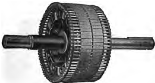
FIG. 1,759. —Western Electric squirrel cage armature. The inductors consist of solid copper bars embedded in the slots of a laminated core, with their projecting ends securely fitted and soldered to heavy copper rings.
