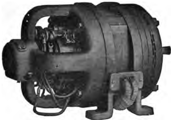
FIG. 1,886.—General Electric 5 H.P., 6 pole adjustable speed single phase compensated repulsion motor. This type is suitable for service requirements demanding the use of a motor whose speed can be adjusted over a considerable range, this speed at a fixed controller setting remaining practically unaffected by any load within the motor's rated capacity. With the controller on the high speed points, the motor possesses an inherent speed regulation between no load and full load of approximately 6 per cent. At the low speed points, under similar load conditions, the speed variation will be approximately 20 per cent. To secure adjustable speed control, the armature circuits employ transformers, whose primaries are excited by the line circuit. The secondaries of these transformers are divided into two sections; the first or "regulating" circuit is placed across the energy brushes; the other section, since it is connected in series with the compensating winding, maintains the high power factor and speed regulation obtained in the constant speed type. The speed range is 2 : 1, approximately one-half of this range being below and one-half above synchronous speed.
