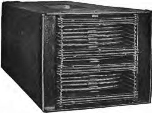
FIG. 1,973.—Assembled coils of General Electric water cooled 500 kva., 66,000 volt transformer.
