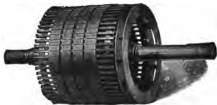
FIG. 1,755. —Western Electric squirrel cage armature of high speed induction motor for centrifugal pump service. This armature is an example of heavy duty construction. The inductors are welded to the short circuiting end rings, the latter being located beneath the inductors, as shown. Fan vanes are provided at one end for ventilation. In the field construction, the core laminations are assembled in a closed box frame, and clamped by heavy rings while under hydraulic pressure. The stator coils are form wound and subjected to a special insulating process, which renders them especially impervious to moisture, and capable of operating without breakdown in locations which are too damp for ordinary motors. The bearing brackets are of rigid mechanical construction, and the pulley end bracket and bearings of all sizes are split to facilitate removal of the rotor and complete inspection. These machines range in size from 50 to 200 horse power, the rugged construction adapting them to heavy and severe service, such as is met with in mining, the construction of dams, canals, aqueducts, tunnels, etc.
