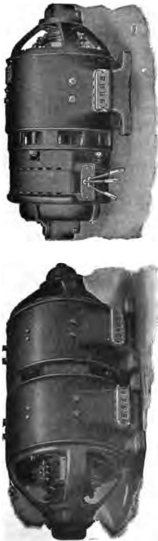
Figs. 2,074 and 2,075. —General Electric charging sets. Fig. 2,074 set consists of dynamo and direct current motor; fig. 2,075 set consists of a dynamo and alternating current motor. Fig. 2,074 set is equipped with 125 volt, shunt wound dynamo and 230 or 550 volt motor and range in capacity from .125 kw. to 13 kw., the speed varying from 2,250 R.P.M. in the .125 kw. set to 925 R.P.M. in the 13 kw. set with 230 volt motor. Both motor and dynamo have the same type and size of frame; these are bolted together and form a compact and symmetrical outfit, no base being necessary. Sets of the type shown in fig. 2,075 range in capacity from .2 kw. to 10 kw. and are equipped with 125 volt shunt wound dynamo and 110, 220, 440 or 550 volt two or three phase motors. If desired they can be furnished with single phase motors wound for 110 or 220 volts. The speed of this type is 1,800 R.P.M. When a motor generator set is used to charge only one battery, the insertion of a resistance between the charging dynamo and the battery is not necessary, inasmuch as all adjustments of voltage can be made by varying the field strength of the dynamo, and, therefore, there are no large losses due to resistance since the loss in the dynamo field rheostat is very small. When a motor generator set is used to charge two or more batteries of different capacities, or voltages, or which are in different conditions of charge, it is necessary to insert a resistance in series with each battery, in order that the current may be properly adjusted for each particular battery.
