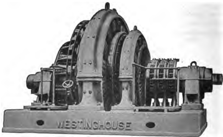
FIG. 2,063. —Westinghouse 2,000 kw., 270 volt, direct current, 6 phase, 167 R.P.M., synchronous booster rotary converter, having a voltage range from 230 to 310 volts. It consists of a standard rotary converter in combination with a revolving armature alternator mounted on the same shaft with the rotary converter and having the same number of poles. By varying the field excitation of the alternator, the alternating current voltage impressed on the rotary converter can be increased or decreased as desired. The direct current voltage delivered by the converter is thereby varied accordingly. The principle of operation of the booster converter is therefore very simple and easily understood. It is simply a combination of two standard pieces of electrical apparatus, accordingly there are incorporated in it no details of construction essentially different from those encountered in standard rotary converters and alternators. The only novelty is in their combination. The frames may be supported either from the rotary converter frame, as in the small units, or from the bed plate, as in the larger ones. A synchronous booster converter can be built, if necessary, with a vertical shaft to satisfy special floor space and head room requirements.
