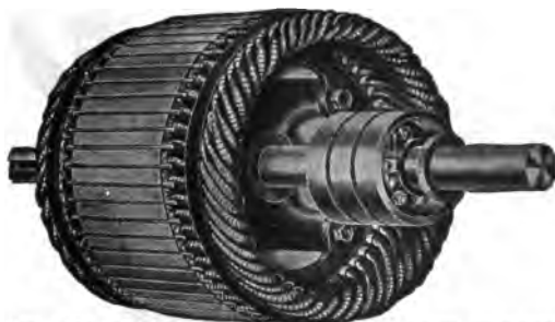
FIG. 1,771.—Richmond slip ring armature as used on motor in fig. 1,770.
