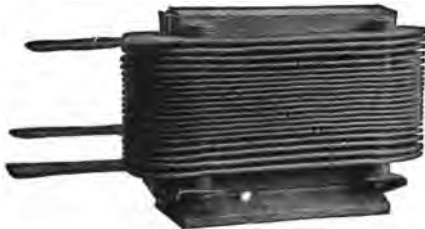
FIG. 2,049. —Commutating pole of Westinghouse commutating pole rotary converter. The commutating poles are similar in general construction to the main poles. The coils are of bare copper strap wound on edge. Ventilating spaces are provided between the pole and coil and between turns. The copper winding is bare except for a few turns at each end. Insulating bolts retain the turns in their proper position.
