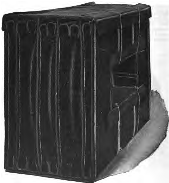
FIG. 1,920.—Wagner coils with insulation ready for core assembly. The flat coils, sometimes called pancake coils, are wound of flat, cotton covered, copper strip with ample insulation between layers. In heavy coils several flat strips in multiple are used per turn in order to facilitate the winding and produce a more compact coil. In many cases normal current flow per high tension coil is very low and could be carried with a very small cross sectional area of copper; however, flat strip is almost always used on account of the increased mechanical stability thus obtained.
