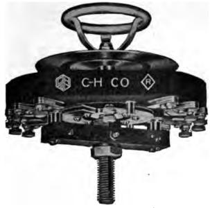
669.—Crouse-Hinds radial ammeter switch, arranged for mounting directly on the itchboard. It is designed for use with external shunt ammeters of any make or capacity, 1 in connection with the required number of shunts, makes possible the taking of current dings of a corresponding number of circuits by means of one ammeter. The wiring gram is shown in fig. 2,670.
