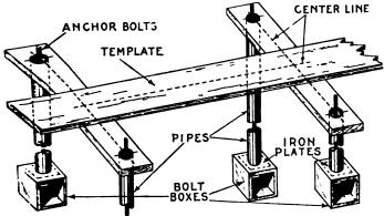
2.735.—View showing part of template for locating anchor bolt centers, pipes through which the bolts pass and bolt boxes at lower end of bolts. The completed foundation is shown in fig. 2.734, with template removed. The template is made of plain boards upon which the center lines are drawn, and bolt center located. Holes are bored at the bolt centers to permit insertion of the pipes as shown.
