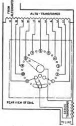
2.436.—Diagram of connections for Westinghouse 11 point dial, series transformer auto-transformer has a number of taps connected acros line, the series transformer is placed in series with one side of the line, and connect a dial, as shown.
