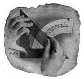
Fig. 2,495.—A calibrated scale. This means that printed scales are not employed, bu instrument has its scale divisions plotted by actual comparison with standards, after the division lines are inked in by a draughtsman. There are makes of direct c instruments employing printed scales in which the scale deflections are fairly ax even though the scales are printed, but printed scales should not be used on alter current instruments.
