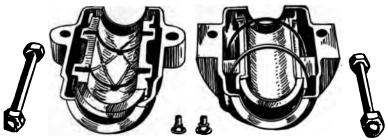
Cs. 2,789 to 2,794.—Self ciling self aligning bearing open. Views showing oil grooves, rings, bolts etc.
