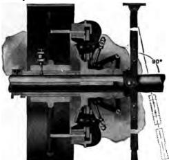
Fr. 2316.—The Hill friction clutch pulley for power control. The clutch mechanism will start a load equivalent to the double belt capacity of the pulley to which the clutch is attached.
