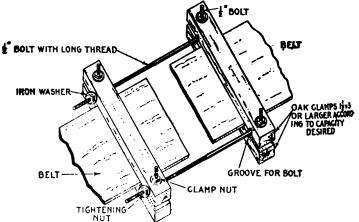
Fig. 2.808.—Home made belt clamp. It is made with four pieces of oak of ample size to find grip the beit ends where the belts are tuchtened. The figure shows the clamp complete and in position on the belt and clearly illustrates the details of construction. In making the long bolts the thread should be out about three-quarter length of bolt and deep enoughs that the mits will carily screw on.
