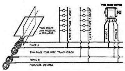
Psc. 2,151.—Diagram of two phase four wire system. It is desirable for supplying current for lighting and power. The arrangement here shown should be used only for lines of short or moderate length, because of the low voltage. Motors should be connected to a circuit separate from the lighting circuit to avoid drop on the latter while starting a motor.
