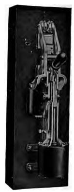
Fig. 2,331.—Condit 600 volt, 1,500 ampere, single pole type K circuit breaker pneumatically operated. It is the same as the electrically operated circuit breaker, except that a pneumatic cylinder mechanism is supplied in place of either the electromagnet or the motor. This cylinder mechanism is so arranged that the air pressure is about the six pressure is about a pressure in a control of the control of the
