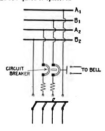
Fig. 2,330.—Diagram showing two phase motor or feeder circuit protected by double coil, overload circuit breaker (or two single pole breakers interlocke alarm switch.
