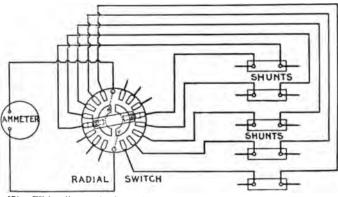
Fig. 2,070.—Wiring diagram for Crouse-Hinds radial ammeter switch as illustrated in fig. 2608. The switch proper is on the rear of the switchboard, and the hand wheel dial and indicator on the front.
