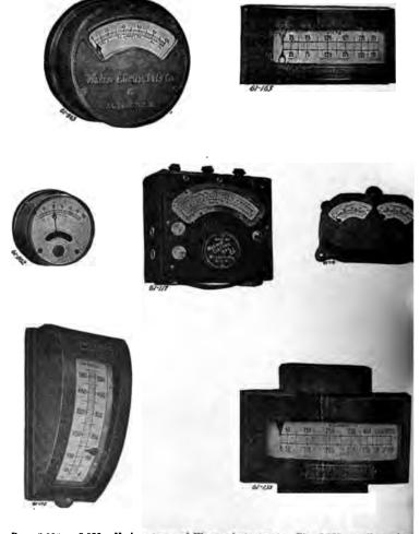
Pics. 2,520 to 2,526.—Various types of Wagner instruments. Fig. 2,520, small round typing. 2,521, horizontal edgewise type; fig. 2,522, smallest switchboard type; fig. 2,523, prable type; fig. 2,524, combination voltmeter and ammeter in one case; fig. 2,525, vets type; fig. 2,526, polyphase type.
