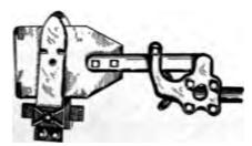
Pm. 2.215.—Pacific swivel type blade for Baum pole top switches. The twist type of blade, here shown, is especially adapted to switches operating in freezing or sleety weather. It will be seen that the first few degrees through which the rotating insulator is moved here the effect of twisting the blade between the shoes of the contact, which breaks any seal descent freezing, or corrollor.
