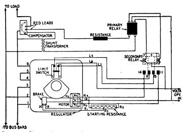
Fig. 2.429.—Diagram of connections of automatic induction regulator and auxiliary appoint on single phase circuit.
