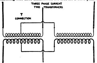
Pic. 2.170.—T connection of transformers in which three phase current is transformed with two transformers. The connections are clearly shown in the illustration. The voltage across one transformer is only 86.6% of that across the other, so that if each transformer be designed especially for its work one will have a rating of .866EI and the other El. The combined rates will then be 1.866 as compared with 1.732 El for three single phase transformers connected either star or delta.
