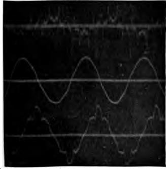
6.2584.—General Electric simultaneous record of three waves with separate zeros.
