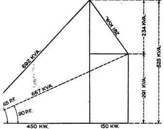
hagram for synchronous condenser calculation for cases where it is desired to energy load with the condenser and still bring the total power factor to .9.
