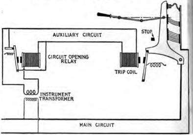
Pig. 2.282.—Diagram illustrating the operation of a circuit opening relay. When the relay contacts are in the normal closed position, as shown, the coil is short circuited. When the predetermined abnormal condition is reached in the main circuit, the relay contacts are opened with a quick break, sending the current through the trip coil momentarily, and opening the breaker.
