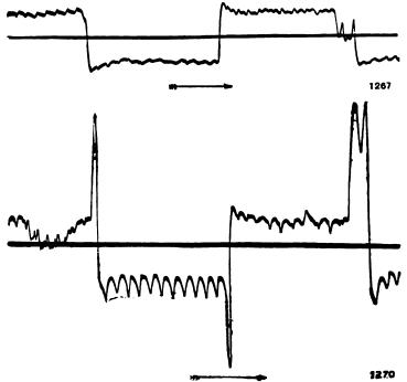
Figs. 2,585 and 2,586.—Oscillograms (from paper by Morris and Catterson-Smith, Proc. I. E. E., Vol. XXXIII, page 1,023), showing how the current varies in one of the armatuse colls of a direct current motor. Fig. 2,585 was obtained with the brushes in the neutral position, and fig. 2,586 with the brushes shifted forward.
