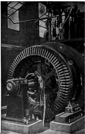
Fig. 2.737. An example of direct connected unit with an engine power. To Westinghouse 200 kvs., 4,000 voit, three phase, 60 cycle alternator direct gas engine.
