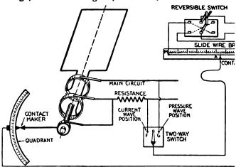
Pig. 2.595.—Diagram illustrating zero method of wave measurement with α. The voltage of the battery must be at least as great as the maximum measured and must be kept constant.
