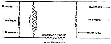
Az. 2.416.—Diagram of induction regulator lowering the voltage 10%. The diagram shows the regulator lowering the feeder pressure to 1,980 volts with an increase of the secondary current to 111 amperes, the additional 11 amperes flowing from the feeder, through the primary back to the feeder.
