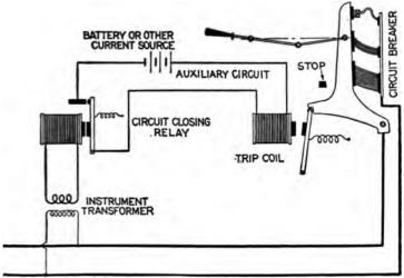
2279.—Diagram illustrating the operation of a circuit closing relay. When the predetermined abnormal condition is reached in the main circuit, the relay closes the auxiliary circuit, thus energizing the trip coil and opening the breaker.
