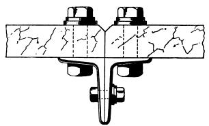
Pig. 2,819.—Method of joining adjacent switchboard panels.
