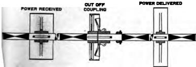
Pa. 2.887.—Cut off coupling for power transmission by line shafting. It is used to cut off a driving shaft from a driven shaft. Its use obviates the use of a quill, such as is shown in fig. 2.868.
