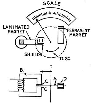
Figs. 2,505 and 2,506.—Plan and elevation of shielded pole type of induction instrum
