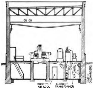
4.2.775.—Plan of sub-station with air blast transformers and motor operated oil switches and underground 11,000 or 13,200 volt high tension lines.
