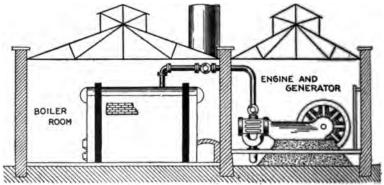
Fig. 2.705.—Elevation of small station with direct drive, showing arrangement of the bolls and engine, piping, etc.
