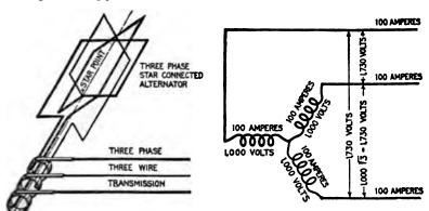
From 2,166 and 2,167.—Three phase star connected alternator, and conventional diagram
