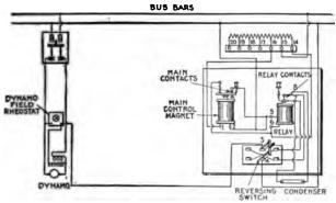
2,428.—Diagram of connections of General Electric direct current (form S) voltage equiator, for 125, 250, and 550 volts. The range of voltage is given in the follow-table:
