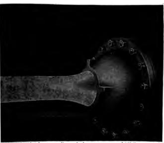
ater discharging from a needle nozzle due to a pressure of 169 lbs. per sq. in.
