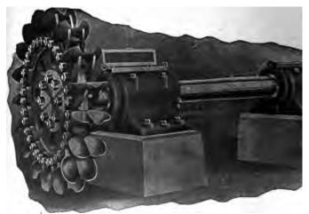
Fig. 2.859.—Single overhung tangential water wheel equipped with Doble ell ets. The central position of the front entering wedge or lip of the bucket the form of a semi-circular notch, which allows a solid circular water jet to d the central dividing wedge of the bucket without being split in a horizonta
