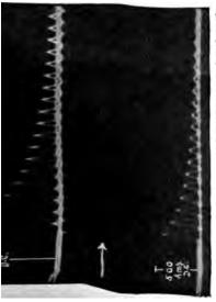
Pro. 2,631.—First rush of current from alternator when short circuited, showing unsymmetrical current wave also wave of field current caused by short circuit current in armature. Upper curve, armature current; lower curve, field current.
