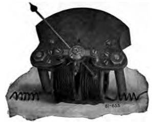
i.—Wagner dynamometer movement. In this type of instrument the deflection is rtional to the square of the current, producing a constantly decreasing sensitiveness: pressure applied is decreased. The dynamometer movement is, for any indication, accurate than the magnetic vane, but cannot readily be employed for the indication rent, as required in ammeters.
