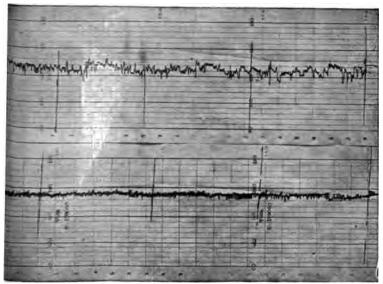
2.483.—Curve drawing voltmeter records at Kennett, Cal. The upper curve shows witage regulation with synchronous condenser out of service, and the lower curve, with synchronous condenser in operation.
