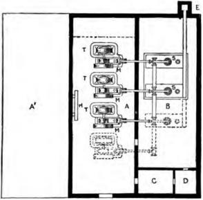
732.—Plan of electrical station containing direct connected units. As shown, space is wided for an extra boiler and engine and generator set, as indicated by the dotted lines are also exists for a storage battery room if necessary, and the partition diding this on from the engine and dynamo room is shown by a dotted line as in previous cases.
