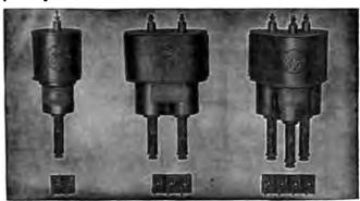
12.224 to 2.329.—General Electric inverse time limit overload circuit closing relays. In this type of relay its mechanism is so designed that a delay or lapse of time in opening the circuit breaker after a pre-determined condition of the circuit has been reached, depends on the flow of current, that is, if the current be great, the time will be small, and if the current be of a moderate value, the time will be correspondingly longer.
