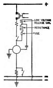
Pig. 2.280.—Diagram showing a railway synchronous converter protected by a single pole overload circuit breaker with low voltage release attachment and bell alarm switch. The low voltage attachment trips the breaker on failure of direct current voltage also what speed limit device closes. Internal troubles are taken care of by the alternating current automatic devices (not shown).
