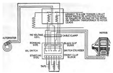
Fig. 2.477.—Diagram of connections of General Electric three phase starting countries with low voltage release and overload relays for 1,040-2,500 volt circuits.
