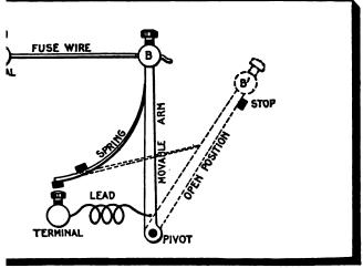
Quick break fuse. The fuse wire is connected between the fixed terminal A novable arm B, and is held under tension by the spring which exerts pressure revable arm in a direction tending to separate A and B. In operation, when the a, the movable arm quickly moves to the position B', thus attenuating the arc crating its extinguishment.
