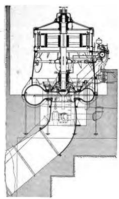
Pig. 2.764.—Sectional elevation of one of the 5.000 horse power vertical Polion-Francis textunes through connected to generator, as installed for the School tady Power Co.
