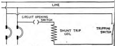
Fig. 2.270.—Diagram of General Electric shunt trip with auxiliary circuit opening, switchly throw coil out of circuit after tripping.
