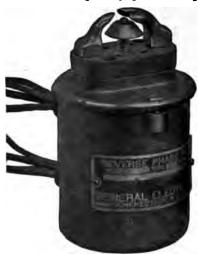
Pig. 2,306.—Alternating current series reverse phase single pole, circuit closing, t relay for 600 volts or less. This type of relay is used chiefly to open motor elevators to prevent damage in case of reversal of leads in reconnecting win or three phase motors. The relay is provided with a dust proof metal cover.
