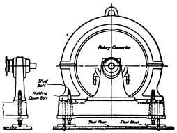
Pigs. 2,782 and 2,783.—Views of levelling device for Westinghouse converter.
