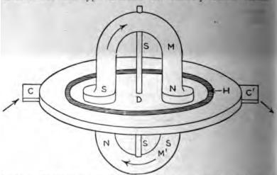
Pig. 2,558.—Faraday disc, or mercury motor ampere hour meter; view showing electric and magnetic circuits.
