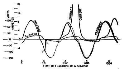
Fig. 2.626.—Curves reproduced from an article by J. T. Morris in the *Electrician*. "On recoming transitory phenomena by the oscillograph."
