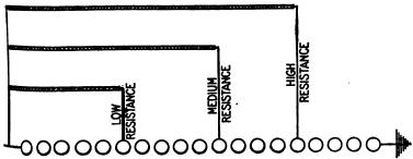
Fig. 2358.—Arrangement of graded resistances on multigap arrester.
