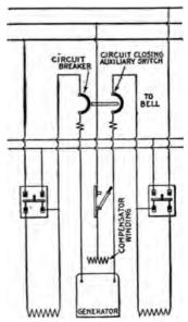
48.—Diagram showing three wire dynamo protected by double pole double coil overl circuit breaker (or two single pole breakers with interlock) with bell alarm switches. splete protection is secured as breaker is connected between armature and series field.
