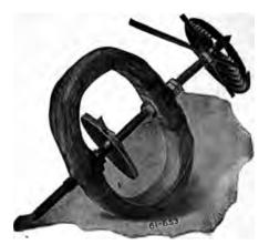
Pic. 2.515.—Armature of 'dynanometer movement.' accuracy is claimed for this ment than the magnetic vait cannot readily be empk the indication of current required in ammeters. The netic vane movement on the A. C. ammeter, and used also in the A. C. volt it makes use of its conspring only for the purposisting the pull on the vather returning of the poisero. The dynanometer ment is recommended for meters.
