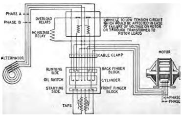
F10. 2.465.—Diagram of connections of General Electric two phase starting competers with no voltage release and overload relays for 1,040 to 2,000 volt discults.
