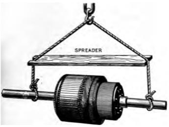
bc. 2.798.—View of armature in transit showing use of a wooden spreader as a protection. If a chain be used in place of the rope, a padding of cloth should be placed around the armature shaft and special care taken that the chain does not scratch the commutator.
