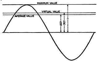
491.—Line curve of alternating current, illustrating various current or pressure values, be virtual value, or .707 × maximum value, is the value indicated by an ammeter or volteter. Thus, if the maximum value of the current be 100 volts, the virtual value as indited by an ammeter is 100 × .707 = 70.7 amperes.
