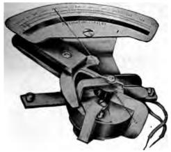
12.—Hoskins instrument with case removed. It has a very short magnetic circuit ich is composed of silicon steel, permitting low magnetic densities to be used.
