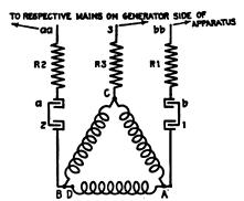
SCHEME OF 3 PHASE NO VOLTAGE CONNECTIONS
