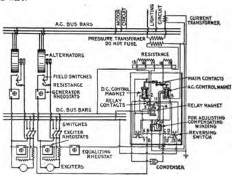
Fig. 2,830.—Diagram of switchboard connections for General Electric automatic we regulator with two exciters and two alternators.
