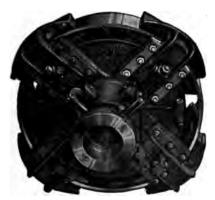
2.818.—Hill clutch mechanism Smith type. The friction surfaces are wood to iron, the
