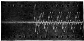
868. 2.624.—Portion of oscillograph record taken with cinematograph film camera, showing the rush of current and sudden rise of voltage at the moment of switching on a high tresture feeder.
