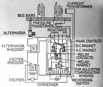
Fro. 2,839.—Diagram of connections of General Electric voltage regulators for one or alternators using one exciter.
