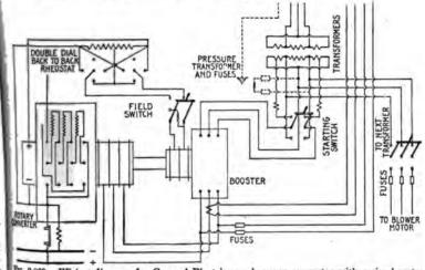
No. 2,869.—Wiring diagram for General Electric synchronous converter with series booster as illustrated in fig. 2,863.
