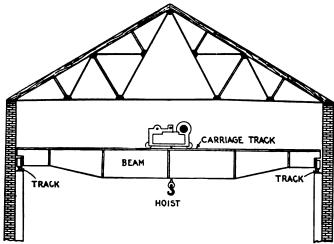
ic. 2.796.—Cross section of electrical station showing small traveling crane.
