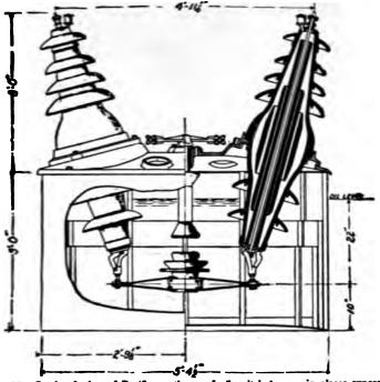
E. 2.221.—Sectional view of Pacific weatherproof oil switch for use in places exposed to the weather. All moving and contact parts are supported from the cast iron top and are readily removable for inspection or repair
