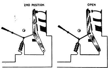
Figs. 2.250 to 2.253.—Elementary diagrams illustrating the operation of a carbon circuit breaker of the overload type, showing the progressive opening of such device. Fig. 2.250, closed position; fig. 2.251, main contacts open; fig. 2.252, intermediate contacts open; fig. 2.253, carbon contacts open, circuit broken.
