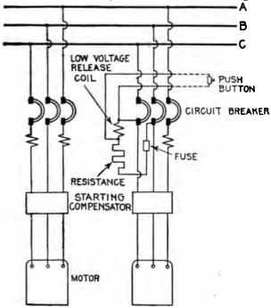
2.281.—Diagram showing three phase motors protected by triple pole overload circuit seakers, with two overload coils, also one overload coil and low voltage release coil. The seaker to be tripped from a distance by means of a short circuiting switch or push button.
