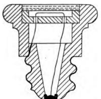
Fig. 2.239.—Cross section through plug fuse. With this type of fuse it is impossible to place any except the correct size of plug in the socket.
