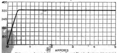
2.301.—Volt ampere characteristic curve of a General Electric aluminum (electrolytic) cell on alternating current. The permanent critical voltage is between 335 and 360 volts. With alternating current, the cell acts as a fairly good condenser, and there is not only the leakage through the film, but also a capacity current flowing into the cell. The phase of this current, then is nearly 90 degrees ahead of the pressure and represents a very low energy factor.
