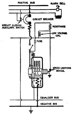
Fig. 3.073.—Diagram of connections of General Electric low voltage release coil wh with speed limiting device on rotary converter.
