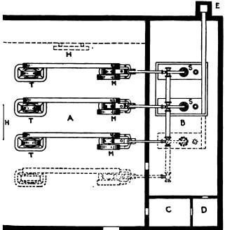
l.—Plan of electrical station with belt drive without counter shaft. The installation represented consists of two boilers, S, etc., and three sets of engines and generators, etc. Sufficient allowance has been made in the plans, however, for future increase sness, as additional space has been provided for an extra engine and generator set, licated by the dotted lines.
