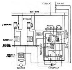
.—Diagram of connections of General Electric direct current voltage regulator T) with two dynamos and one exciter. In cases where several shunt or compound d direct current machines are operating in parallel, either on two wire or three wire ms, a good arrangement for voltage regulation and line drop compensation is ned by using this regulator and a separate exciter. The compensating shunt as well sesure wires can be used to maintain a constant pressure at the center of distribution.
