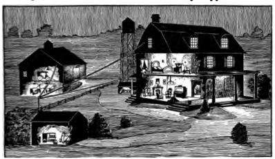
Pig. 2,145.—View of a typical isolated plant. The illustration represents an electric lighting plant on a farm showing the lighting of the dwelling, barn, tool house and pump house. The installation consists of a low voltage dynamo with gas engine drive and storage battery together with the necessary auxiliary apparatus.
