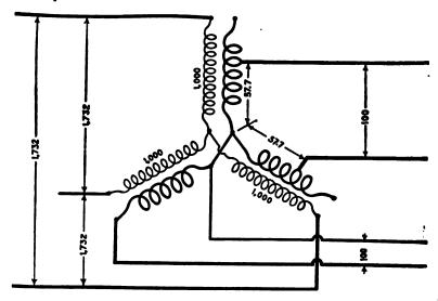
Fig. 2.177.—Three phase to two phase transformation with three star connected transformata. Two of the secondary windings are tapped at points corresponding to 57.7% of full voltages these two windings are connected in series to form one secondary phase of voltage equal to that obtained by the other full secondary winding.
