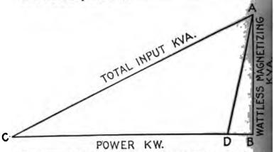
Prc. 2.478.—Diagram showing relative effect of fully loaded and lightly loaded induction metro on power factor.
