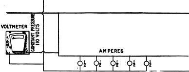
Fig. 2,136.—Diagram of parallel circuit. It is a constant pressure circuit and is very widely used for lighting and power: If each lamp take say 1/2 ampere, the current flowing in the circuit will vary with the number of lamp in operation; in the above circuit with all lamps on, the current is 1/2 × 5 = 21/2 amperes.
