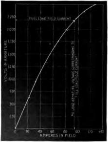
Ftc. 2.785.—Saturation curve taken from a 2,000 kw., three phase alternator of the field type, having 16 poles, and generating 2,000 volts, and 576 amperes per ph run at 300 R.P.M.
