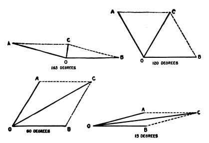
Pros. 2,125 to 2,128.—Parallelograms of forces showing increase in magnitude of the resultant of two forces, as their difference of direction, or electrically speaking, their phase difference is diminished. The diagrams show the growth of the resultant of the two equal forces OA and OB as the phase difference is reduced from 165° successively to 120, 60, and 15 degrees.
