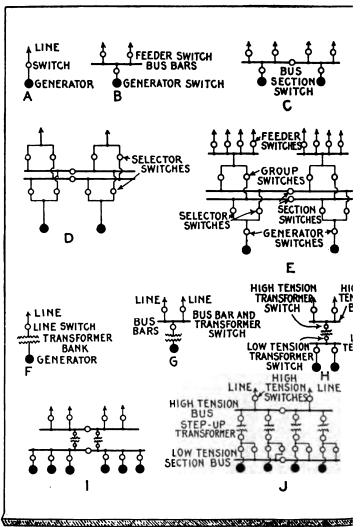
Figs. 2,645 and 2,646. - Diagrams illustrating general principles of switchboard connection
