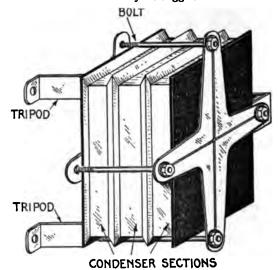
Fig. 2,452.—Condenser sections and method of assembling same with tripod. Ti bolts are made of extra length to accommodate the addition of extra condense if necessary. The illustration shows three sections in position.
