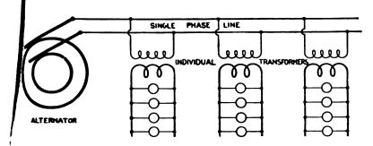
No. 2.139.—Diagram of transformer system with individual transformers. The efficiency is low, but such method of distribution is necessary in sparsely settled or rural districts.
