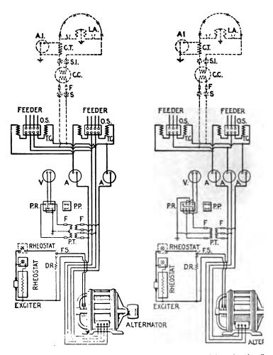
Figs. 2,667 and 2,668.—Diagrams of connections for two phase and three phase install A and A1, ammeter; C.C., constant current transformer; C.T., current transformer, discharge resistance; F, fuse; F.S., field switch; L.A., lightning arrester; O.S., oil P.P., pressure plug; P.R., pressure receptacle; P.T., pressure transformer; S and S switches; T.C., oil switch trip coil; V, voltmeter.
