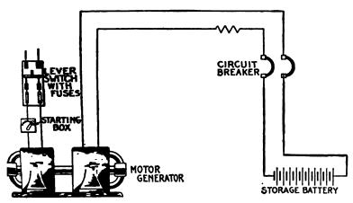
Pt. 2344.—Diagram showing storage battery and charging dynamo protected by double pole single coll underload circuit breaker. In operation, the circuit breaker disconnects the battery when fully charged, and protects the dynamo from reverse current.
