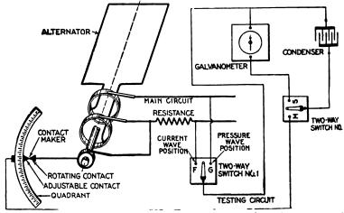
Pig. 2,589.—Diagram illustrating Joubert's step by step method of wave form measurement
