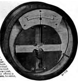
Pig. 2,580.—Westinghouse single phase electrostatic ground detector.
