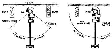
Figs. 2,786 and 2,787.—Wheel and roller pipe cutters illustrating range. The illustration. The wheel cutter requiring only a small arc of movement will cut a prinaccessible place as shown, which with a roller cutter would be impossible. Acc the wheel cutter is said to have a greater range than the roller cutter.
