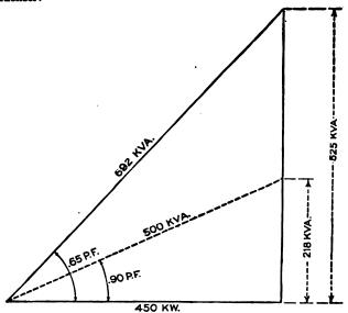
Fig. 2,488.—Diagram for synchronous condenser calculations.
