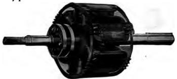
Pic. 2.481.—Field of a synchronous condenser Note the amortisseur winding, erroneously called equirrel cage winding, consisting of two end rings which serve to short circuit spokes passing through the pole tips as shown. The amortisseur winding assists in starting and serves also as a damping device to minimize hunting.
