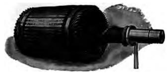
ht. 2.418.—Moving element or primary of Westinghouse motor operated polyphase induction regulator.
