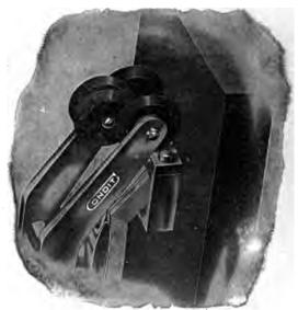
Pic. 2,248.—Carbon break discs of Condit circuit breaker. The two pairs of similar discs which slide past each other are so arranged that these surfaces coincide at the instant the intermediate contact separate after which, as the contact arm opens further, they gradually disengage.
