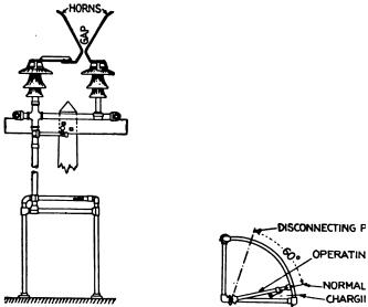
Pics. 2,383 and 2,384.—Elevation and plan of General Electric horn gaps a stand for high voltage arresters.
