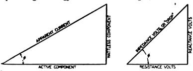
Pm. 2.694.—Diagram showing that the apparent current is more than the active current, the excess depending upon the angle of phase difference.
