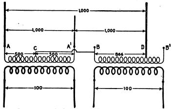
R. 2.176.—The Scott connection for transforming from three phase to two phase. In this method one of the primary wires B of the .866 ratio transformer is connected to the middle of the other primary as at C, the ends of which are connected to two of the three phase wires. The other phase wire is connected at D, the point giving the .866 ratio. The secondary wires are connected as shown.
