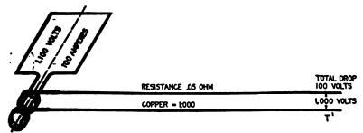
Fra. 2.188.—Single phase line, used as basis of comparison in obtaining the relative weights of copper required by polyphase systems, as indicated in figs. 2,181 to 2,188.
