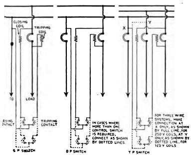
cs. 2,233 to 2,235.—Diagrams showing connections for General Electric single, double, and triple pole, solenoid operated remote control switches. The operating coils are shown connected to main switch circuit, but may be connected to an entirely separate control circuit. Connections are the same for either alternating or direct current.
