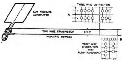
Fig. 2.143.—Diagram illustrating single phase two wire transmission and three wire distribution. The simplified three wire arrangement at A, is not permissible except in cases of very little unbelsacing. Where the difference between loads on each side of the neutral may be great some form of balancing as an auto-transformer or equivalent should be used, as at B.
