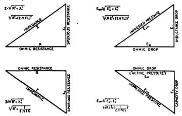
is. 2,689 to 2,692.—Triangles for obtaining graphically, impedance, impressed pressure, etc., in alternating current circuits. For a full explanation of this method the reader is referred to Guide 5, Chapter XLVII or. Alternating Current Diagrams. A thorough study of this chapter is recommended.
