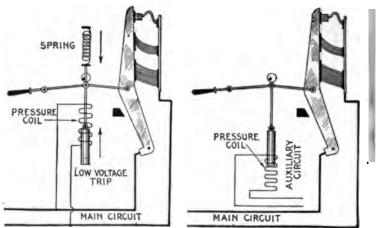
Figs. 2,259 to 2,262.—Elementary diagrams illustrating the various methods of electromagnetic control for circuit breakers. Fig. 2,259, overload trip; fig. 2,260, underload trip, fig. 2,261, low voltage trip; fig. 2,262, control from auxiliary circuit by means of a "relay."
