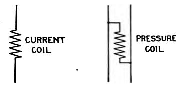
t. 2,267 and 2,268. - Positions in circuit of current and pressure coils of circuit breakers.
