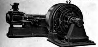
2771.—Direct connected direct current unit with Ridgway high speed four valve engine,
