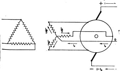
As 2870.—Wiring diagram for three wire synchronous converter with delta-Y connected step down transformer with the neutral brought out. It is evident that in this case each transformer secondary receives 1/2 of the neutral current, and if this current be not so small, as compared with the exciting current of the transformer, it will cause an increase in the magnetic density.
