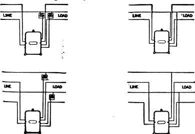
Pics. 2,53 to 2,541.—Connections of Port Wayne multi-phase watt hour meters (type kinoms MAB and MAK), for 100-625 volt circuits, 5-150 amperes. Fig. 2,538 two and three phase, three wire circuit, 25-36 cycles; fig. 2,539 two and three phase, 3 wire circuit, 36 cycles and above; fig. 2,540, two phase 4 wire circuit, 25-36 cycles; fig. 2,541 two phase, 4 wire circuit 36 cycles and above.
