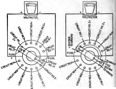
Figs. 2,640 and 2,650,—Wiring diagrams of Crouse-Hinds voltmeter and ground detector switches. Fig. 2,649 voltmeter switch; fig. 2,650 voltmeter and ground detector switch. A view of the switch is shown in fig. 2,648; it is designed for use on two or three wire systems up to 300 volts.
