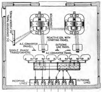
Fig. 2,776.—Plan of small sub-station with single phase oil insulated self-cooling transforms and hand operated oil switches 11,000 or 13,200 volts, overhead high tension lines.
