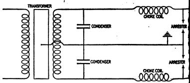
Fig. 2.413.—Diagram showing connections of static interrupter for protecting a transform
