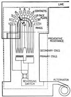
2.—Diagram showing connections of the Stillwell regulator.
