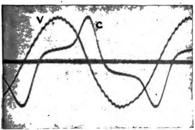
268. 2.593 and 2.594.—Two curves representing previous and current respectively of a retriventively. Fig. 2.593, pressure wave V, fig. 2.594 current wave C. The accesses were obtained from a converter which was being driven by on after one to be a converted on independent motor. The rotary converter was supervised if converted to the representation of teeth in the armature of the rotary converter.
