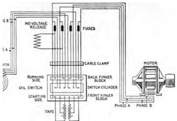
63.—Diagram of connections of General Electric two phase starting compensus with no voltage release and fuses.
