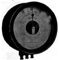
c. 2.567.—Westinghouse induction type frequency meter. The normal frequency is usually at the top of the scale to facilitate reading. The damping disc moves in a magnetic field, thus damping by the method of eddy currents. The standard meters are designed for circuits of 100 volts nominal and can be used for voltages up to 125 volts. For higher voltages, transformers with nominal 100 volt secondary should be used.
