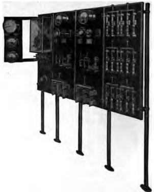
Fig. 2,647.—General Electric small plant alternating current switchboard, designs in small central stations and isolated plants. They are for use with one set of bust which all generators and feeders are connected by means of single throw lever switcircuit breakers, suitable provision being made for the parallel operation of the generators.
