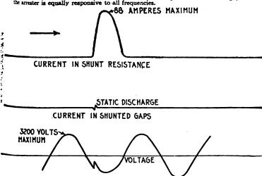
hos 2,353 to 2,355.—Oscillograph record of the phenomena that take place in the different circuits or selective paths of a multi-gap arrester during a discharge such as shown in fg. 2,326.
