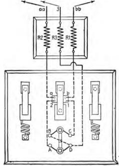
2 PHASE 3 WIRE NO VOLTAGE CONNECTIONS
