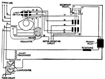
2.430.—Diagram of connections of automatic induction regulator and accessory apparatus on three phase feeder circuit.
