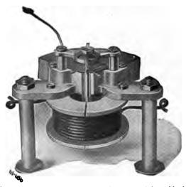
Fig. 2,500.—Magnetic vane movement of a Wagner instrument; it is used both for and ammeters. This type differs from the dynamometer movement in that a vasoft iron replaces the moving coil. The magnetic vane movement makes use a trolling spring only for the purpose of resisting the pull on the vane and the return needle to zero. The spring does not carry any current.
