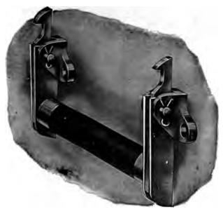
1c. 2,249.—Mechanically connected insulated latches used on Condit circuit breakers to produce inter-locking tripping.
