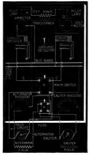
Pic. 2,820.—Switchboard wiring for a single phase separately excited alternator. The direct current circuits are represented by dotted lines, and the alternating current circuit, by solid lines.
