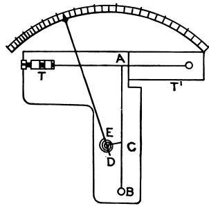
Pa. 2.504.—Diagram illustrating the principle of hot wire instruments. The essential parts are the active wire A, stretched between terminals T and T', tension wire C, thread E, and pulley D to which is attached the pointer.
