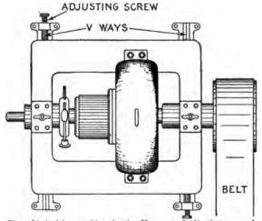
Pig. 2,799.—Plan of belt drive machine showing V ways and adjusting screws for machine forward from the engine or counter shaft to take up slack in the belt.
