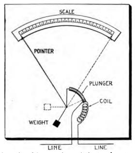
!.—Plunger form of electromagnetic or moving iron type of ammeter.
