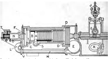
Fig. 2,752.—Sectional view of governor of the Parsons-Westinghouse turbine.
