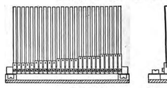
Pros. 2.565 and 2.566.—Side and end views of Frahm resonance type frequency meter reeds. Owing to the principle employed in the meter it is evident that the indications are independent of the voltage, change of wave form, and external magnetic fields.
