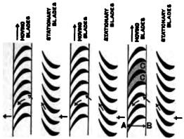
49.—Arrangement of blading in Parsons type turbine, consisting of alternate moving stationary blades. The path taken by the steam is indicated by the arrows
