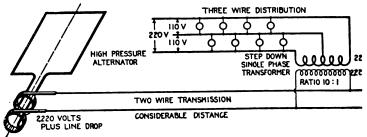
FIG. 2,146.—Diagram showing arrangement of single phase system for two wire transt and three wire distribution, where the transmission distance is considerable. In to reduce the cost of the transmission line, the current must be transmitted at hig sure; this necessitates the use of a step down transformer at the distributing as shown in the illustration.
