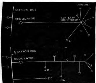
12. 2.706.—Diagram illustrating graphical method of determining the center of gravity of a system in locating the central station.
