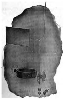
7.—Moving element of Keystone dynamometer instrument. The illustration shows movable coil, pointer, aluminum air vane for damping the oscillations, controlling a, and counter weights.
