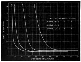
Frg. 2,343.—Characteristic curves of Condit time limit relay as illustrated in fig. 2,342. tings: curve A, 5 amperes; curve B, 6 amperes; curve C, 8 amperes; curve D, 12 amp
