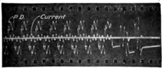
6, 2.625.—Portion of oscillograph record taken with a cinematograph film camera showing the effect of switching off a high pressure feeder and illustrating the violent fluctuations produced by sparking at the switch contacts.
