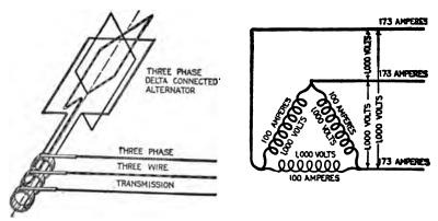
Pics. 2.168 and 2.169.—Three phase delta connected alternator and conventional diagram showing pressure and current relations.
