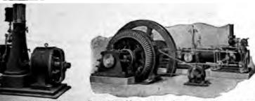
2,769.—Triumph direct rent generator set with right slide valve engine.
