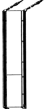
Fig. 2,836.—Method of supporting the framework of a switchboard.
