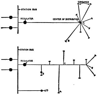
Pics. 2.447 and 2.448.—Systems of distribution illustrating use of small feeder or polyoltage regulators.
