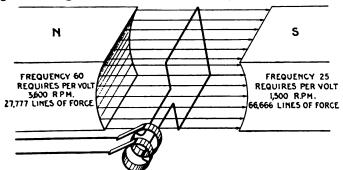
Fig. 2,149.—Blementary alternator developing one volt at frequencies of 60 and 25, showing the effect of reducing the frequency. Since for the same number of pole, the R.P.M. have to be decreased to decrease the frequency, increased flux is required to develop the same voltage. Hence in construction, low frequency machines require larger magnets, increased number of turns in series on the armature coils, larger exciting units as compared with machines built for higher frequency.
