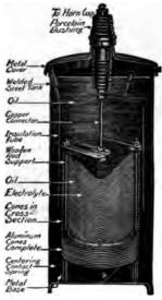
is section of General Electric aluminum (electrolytic) lightning arrester.
