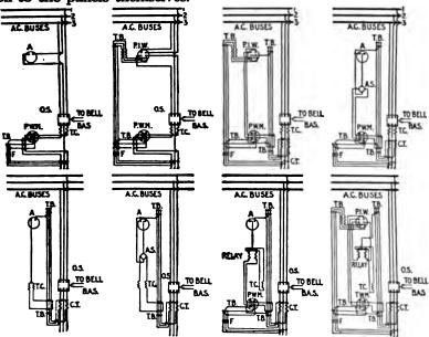
Pics. 2,659 to 2,666.—Diagram of connections for three phase feeder panels. Key to symbols:
