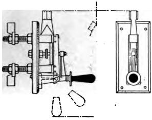
Fig. 2.347.—Thermal overload circuit breaker. In construction two contact blocks are fixed rigidly to, but insulated from the switch arm. They are connected electrically by two parallel strips of suitable metal, each fitted with a steel catch piece. When the switch is closed the strips are sprung apart over a fixed catch, and the full rated current does not release the catch. Overload causes the strips to move apart, and the circuit breaker flies off under the action of a spring.
