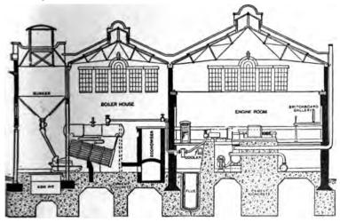
C. 2,710.—Section of the central station or "electricity works" at Derby, showing boiler and engine room and arrangement of bunkers, conveyor, will pit, grates, boilers drum, heating surface and superheater), economizer, flue, turbines, condenser purage, etc.; also location of switchboard gallery and system of piping.
