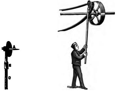
3cs. 2,862 and 2,863.—Method of putting on belts when the driver is in motion, and device used. The latter is called a belt slipper, and consists, as shown in fig. 2,862, of a cone and shield, which revolve upon the stem, B, thus yielding easily to the pull of the belt. A staff or handle C of any convenient length can be fastened to the socket. The mode of operation is illustrated in fig. 2,863, which is self explanatory.
