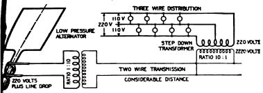
2.2.147.—Diagram illustrating how electricity can be economically transmitted a considerable distance with low pressure alternator already in use.
